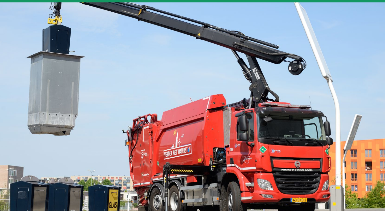
Fuel cell garbage truck in operation since April 2019 in Groningen, NL
