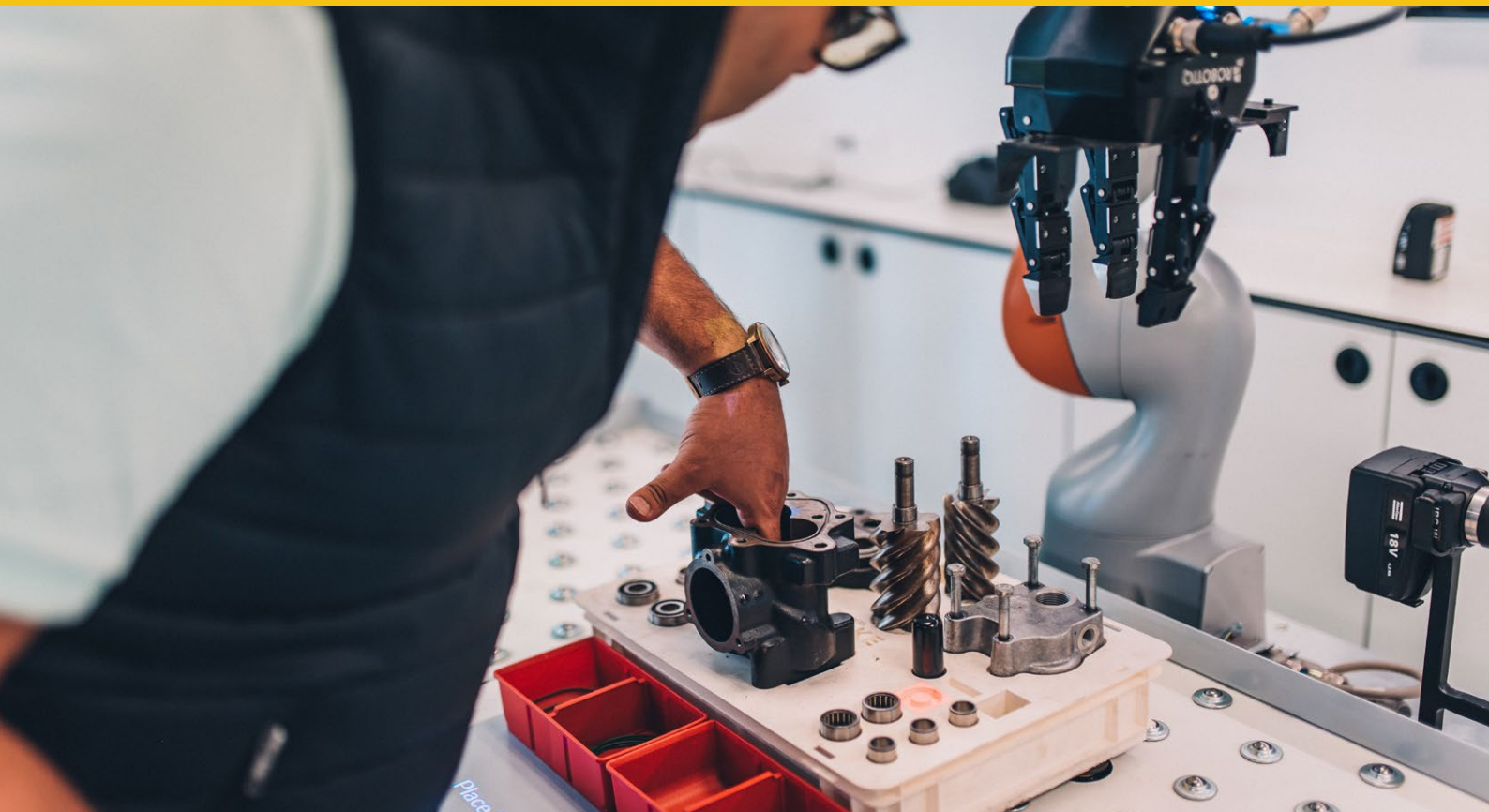
Operator and cobot assembling together an air compressor
