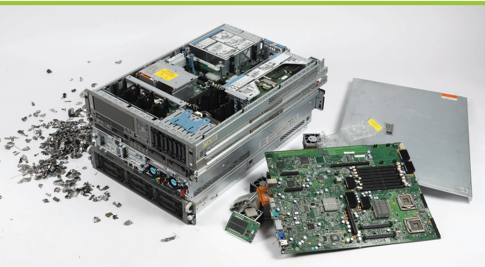
Server disassembly and shredded components
