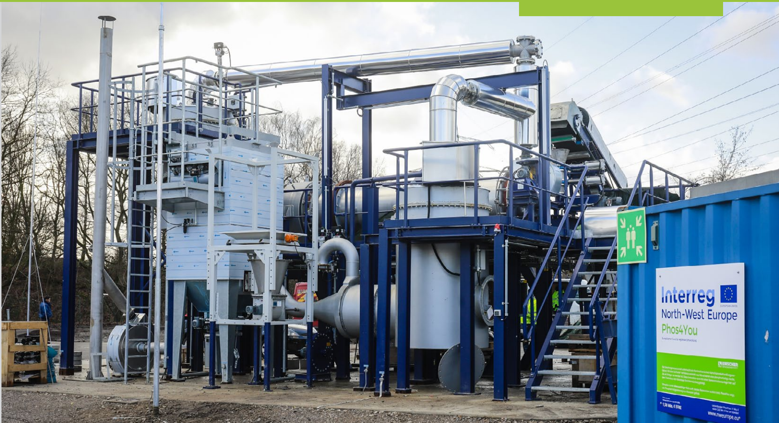
EuPhoRe plant, producing phosphorus rich ashes usable for fertilisers
