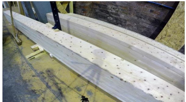
Fig. 7. Dowelled timber beams for the Liverpool demonstrator
