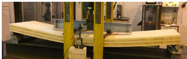
Fig. 2. A DLT panel under four-point bending load (U. Liverpool)
