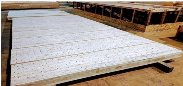
Fig. 1. Dowelled laminated timber (DLT) panels
