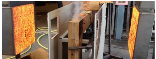
Fire test on L-shaped structure performed at the University of Lorraine
