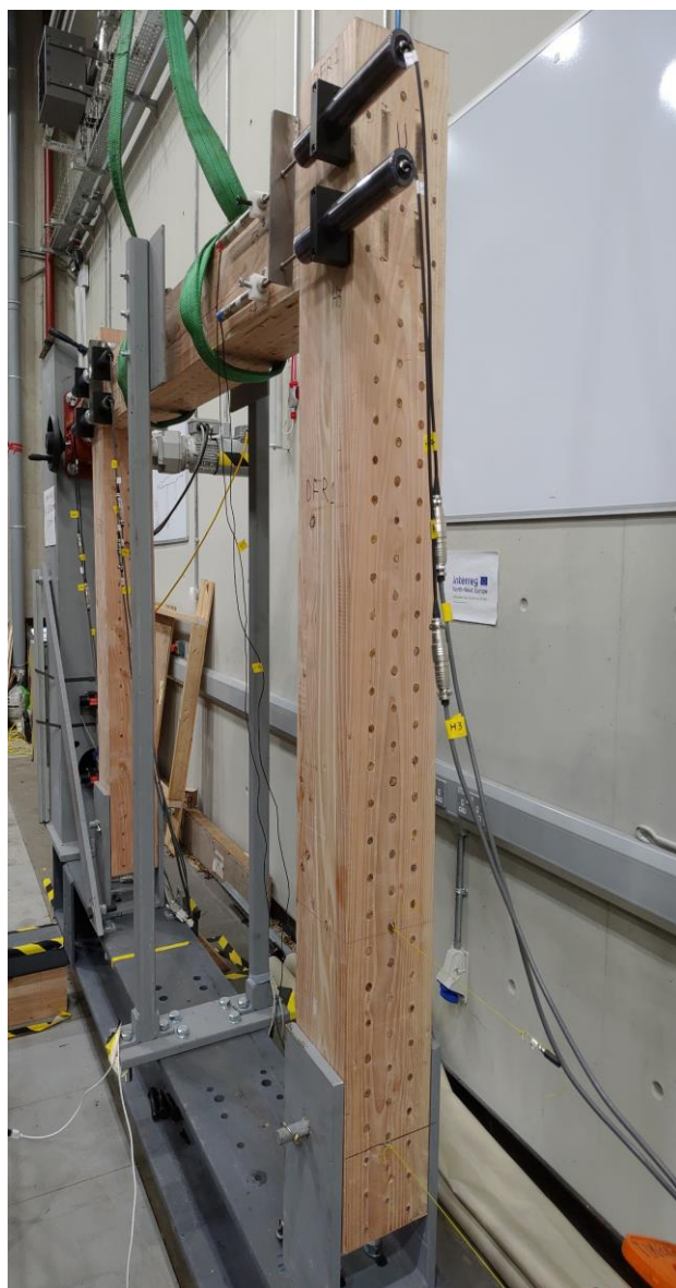
Figure 7 - Testing of adhesive free and non-metallic timber frame
