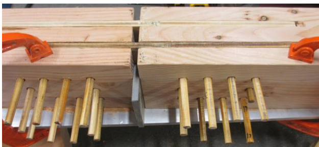
Figure 1 - Orientation of CW connectors in beam-beam connections
