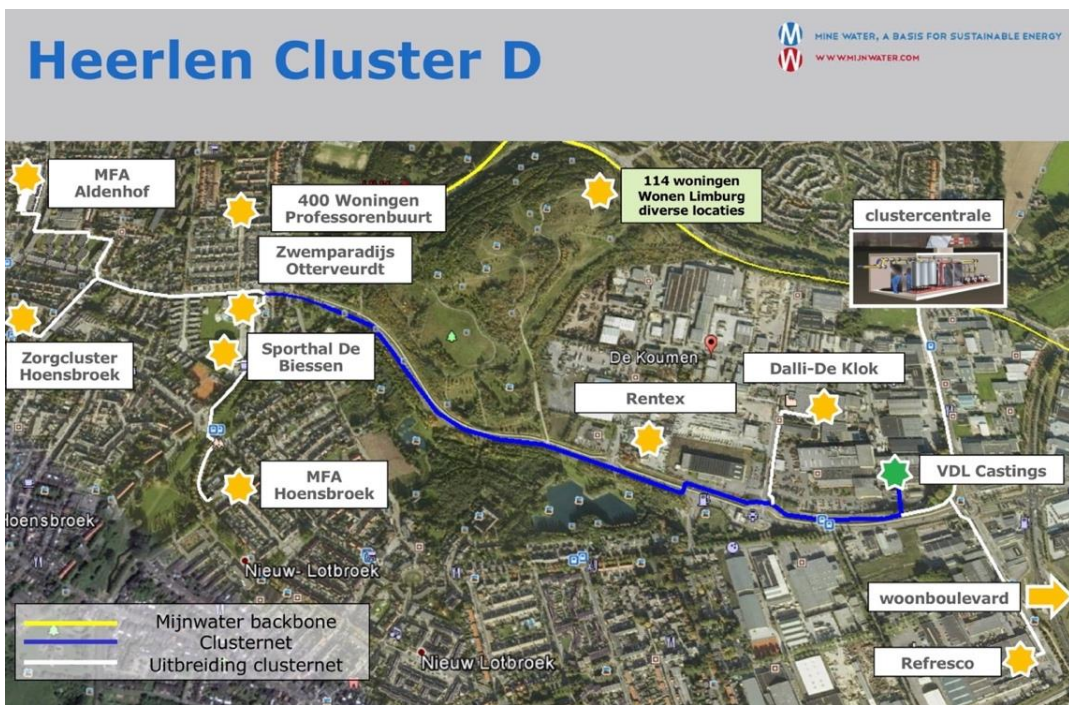
Figure 14: Mijwater Heerlen Cluster D. On the right is the industrial area, on the left an area with residential neighbourhoods, a swimmingpool, a sports centre and a multifunctional centre that are now being connected. The cluster installation connecting with the yellow backbone has just been finished. The green star for VDL Castings was the first industrial partner in this area to get its cooling coupled to Mijwater.
