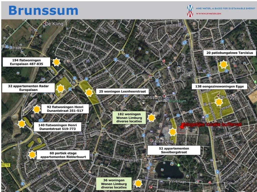
Figure 15: Mijwater Brunssum. Borehole thermal storage is being tested, or created. Work to connect the yellow stars to Mijwater services is to start very soon, starting as an island based on local thermal storage. Connection to the mine water reservoir will happen later.
