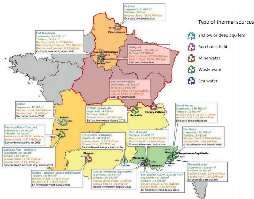
Figure 1. Existing low temperature DHC grids on the national territory and targeted regions for roll-out strategy in red (adapted from AFP, 2019).
