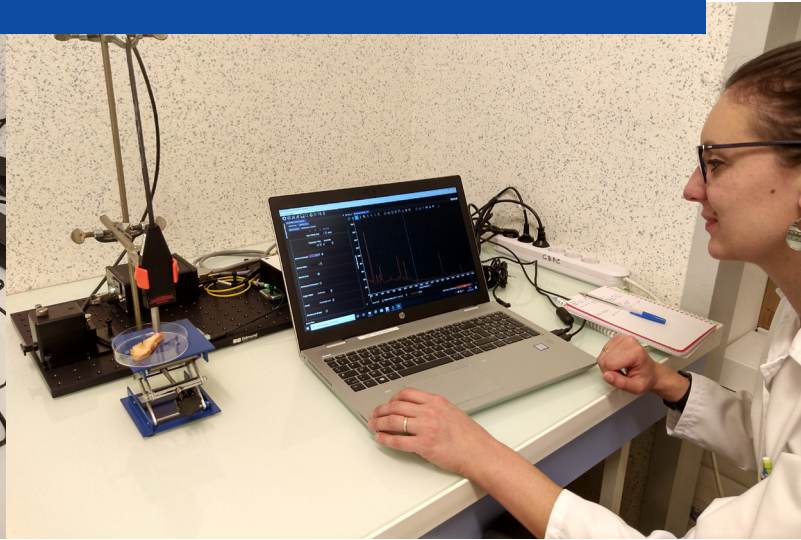
Emilie Grange of the University of Nantes, Using Raman Spectroscopy to test on chicken pieces
