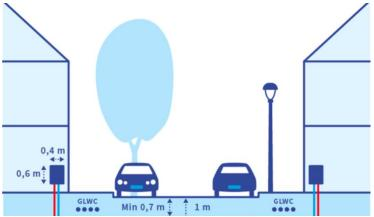
Figure 1-1: general scheme of heatnetwork in a street with gas, electricity, water, communication, sewage
