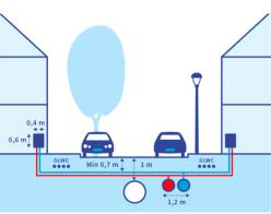
*Lead-up services regulations: regulation for cables and piping* Some cities have preferred profiles for lead-up services or even have lead-up tunnels, in which cables and pipes are combined.
