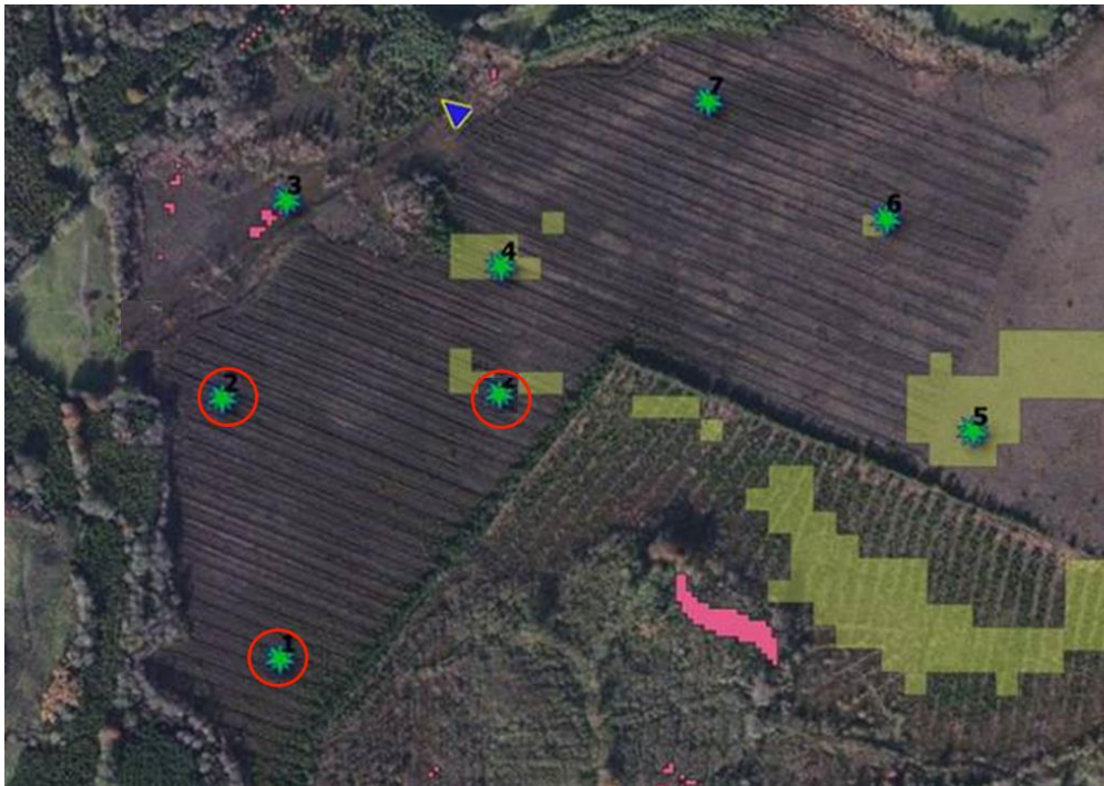
Figure 7 – Site monitoring. Locations with green asterisk are piezometer locations. Locations with red circle are yet to be installed. Blue triangle is a flume to monitor surface water discharge. Yellow polygons represent predicted bog forming areas.
