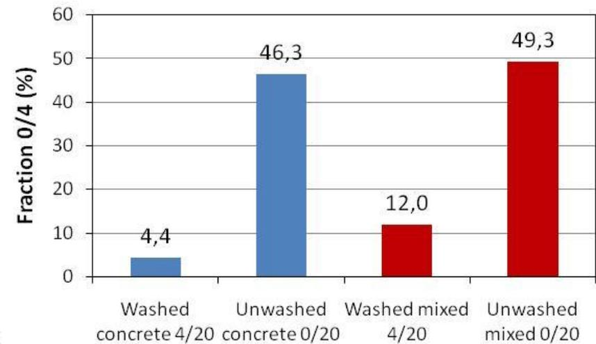
Fine content ( $< 63\mu\text{m}$ ) higher in mixed aggregates and significantly reduced by washing
