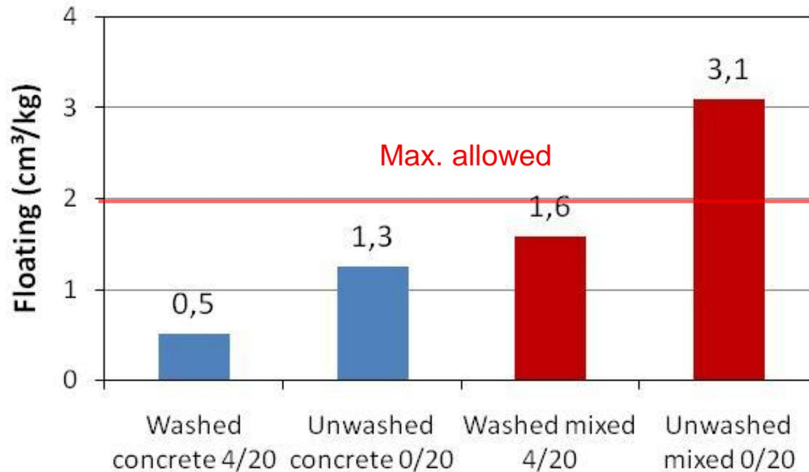
Density decreases with washing due to smaller particles removal but does still fulfill the requirements
