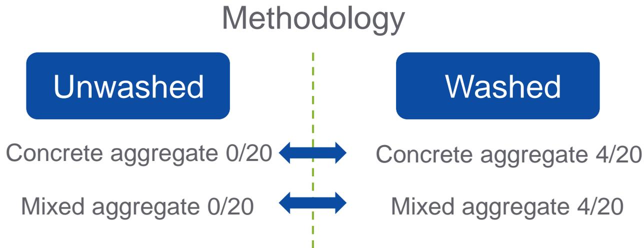
**0/4 fraction comprises nearly 50% of the unwashed aggregates composition**
