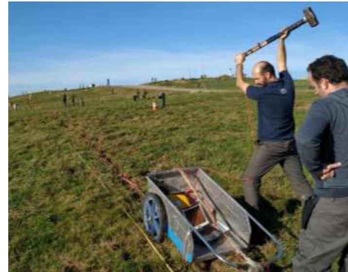
Multi-channel Analysis of Surface Waves (MASW)
