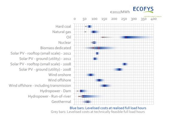
Figure 3: Levelized costs of energy for different technologies for the year 2012 (ECOFYS, 2014). Red lines indicate the median value for the range.
