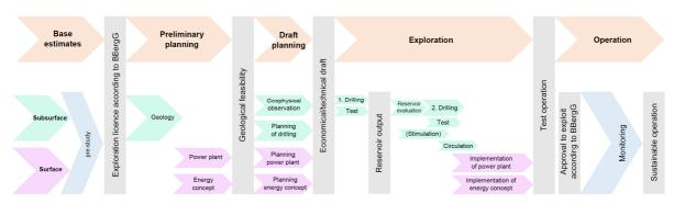
**Figure 1:** Schematic representation of a geothermal project development in Germany (modified after VBI Tiefe Geothermie, 2010). The different stages (orange) can be subdivided in subsurface (green) and surface (purple) investigations.
