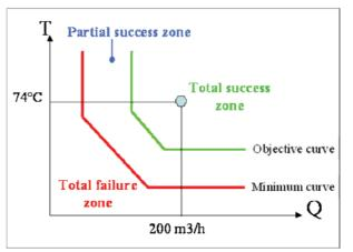
**Figure 5:** Success-failure curve to determine a reliable project (Bézèlgues-Courtade and Jaudin, 2008). Success appraisal is based on the reservoir temperature and flow rate.
