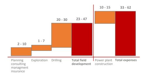
**Figure 2:** Cost range of the development of a 20 MWe convetional high temperature geothermal power plant (Laenen *et al.,* 2019).
