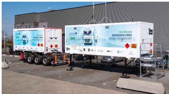
Foto 1: The mobile hydrogen refueling station.
