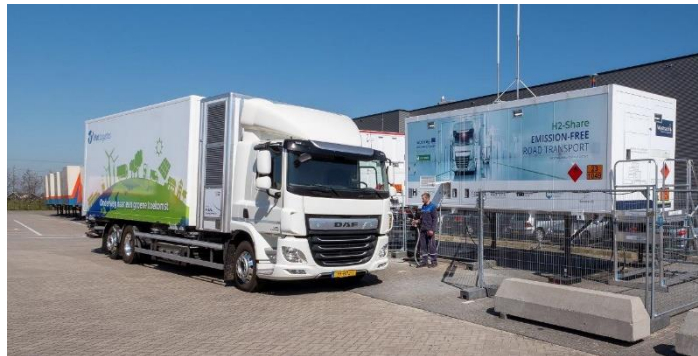
Foto 2: The 27 ton electric rigid truck with hydrogen range extender refueling at the mobile refueler.
