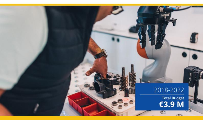
Operator and cobot assembling together an air compressor
