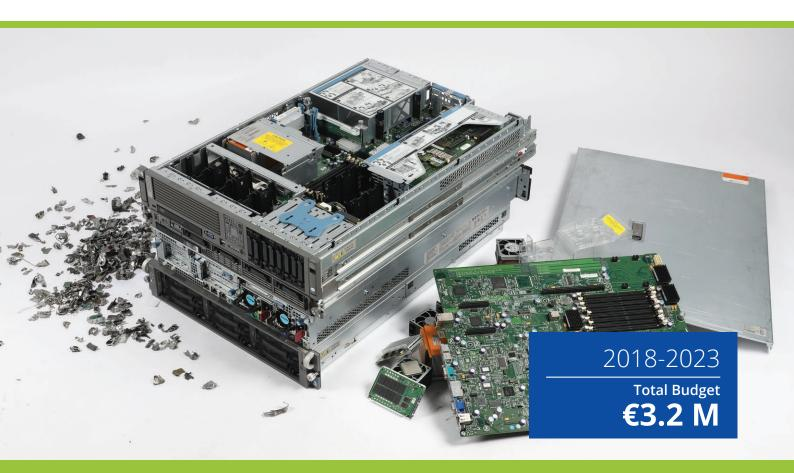
Server disassembly and shredded components
