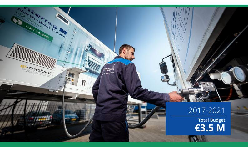
Refuelling the hydrogen truck at the mobile refueler during the first demo at Breytner in the Netherlands
