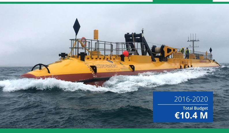
SR2000 device testing at EMEC's Fall of Warness test site
