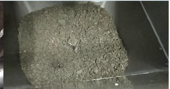
Dewatered cake in the buffer
