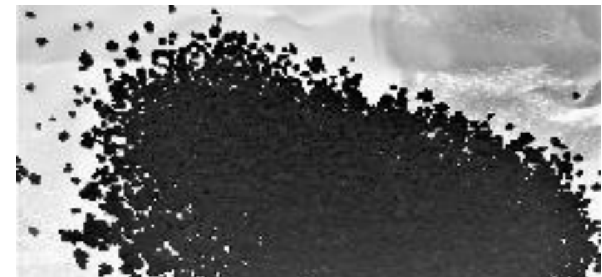
GAC from sewage sludge after pyrolysis
