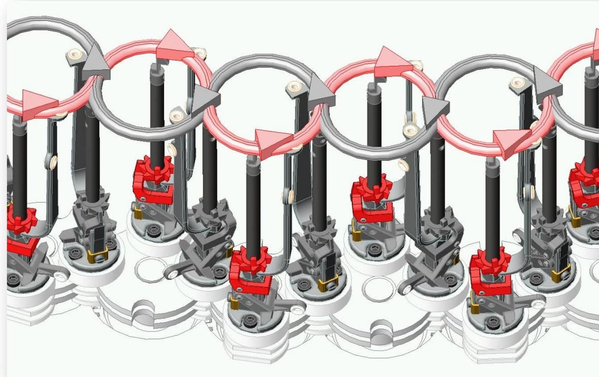
Continuous S motion: clockwise and counter clockwise
