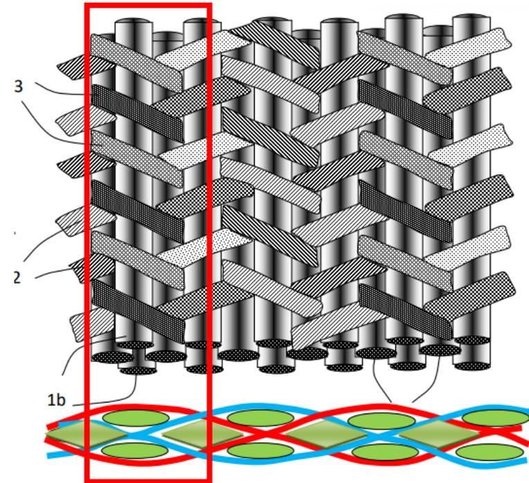
*Innovative braid structure with thickness binding*
