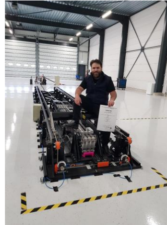
Patented slider system for automatic landing
