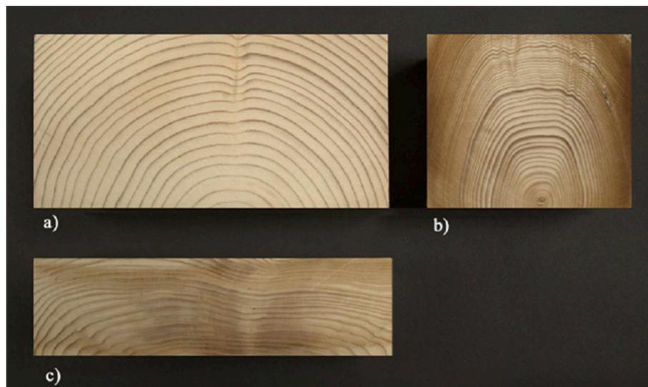
Fig. 1. a) Uncompressed Spruce, b) Compression in the tangential direction and c) Compression in the radial direction [9].
