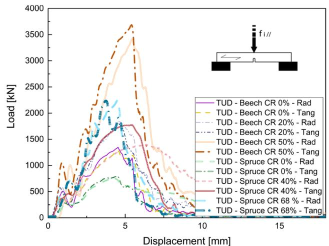
Fig. 12. Average load–displacement curves for Charpy test.
