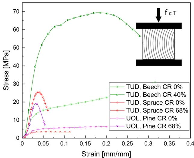
Fig. 6. Average stress–strain compression test curves in the tangential direction.
