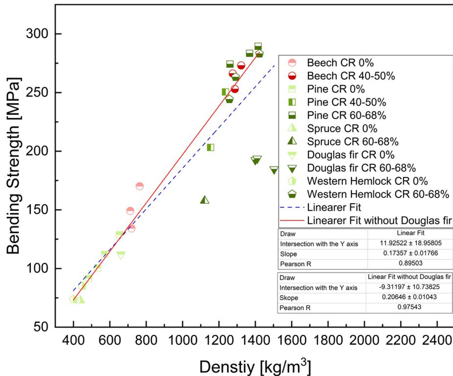
Fig. 13. Flexural strength-density correlation.
