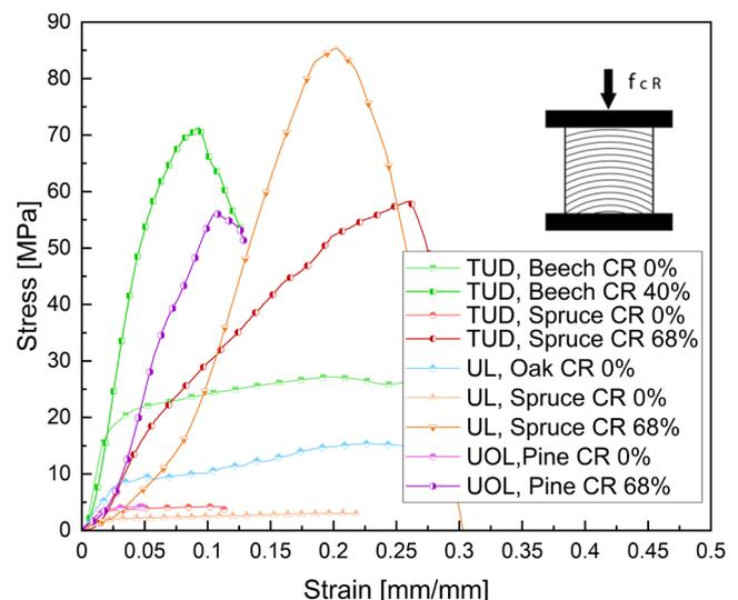
**Fig. 5.** Average stress–strain compression test curves in the radial direction.
