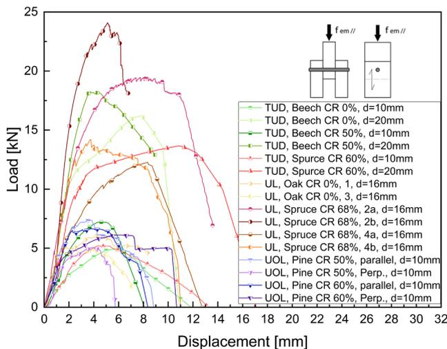
Fig. 11. Average load-slip curves of the push-out shear tests.
