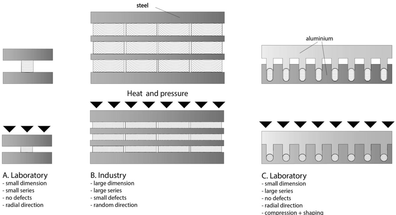
Fig. 3. Different manufacturing setups for compressed wood production.
