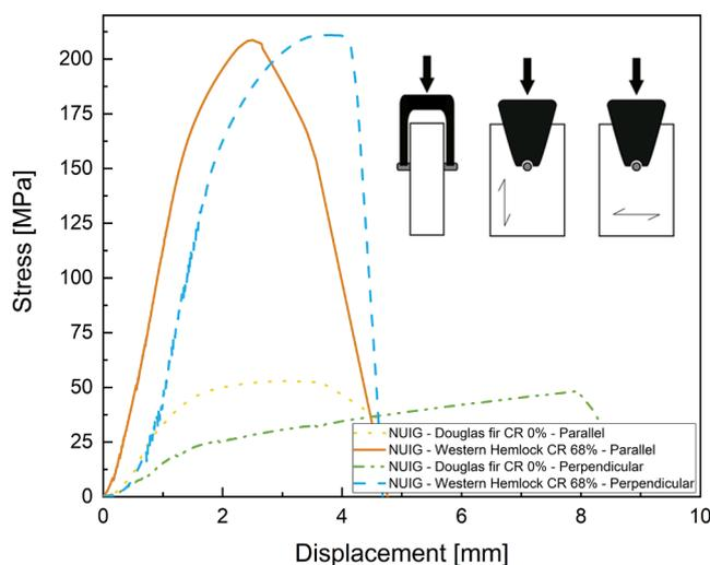
Fig. 9. Average load–displacement curves for the embedment test.
