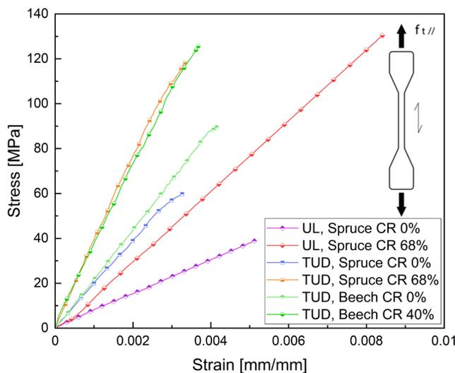
Fig. 7. Average stress–strain curves for tension parallel to the grain.
