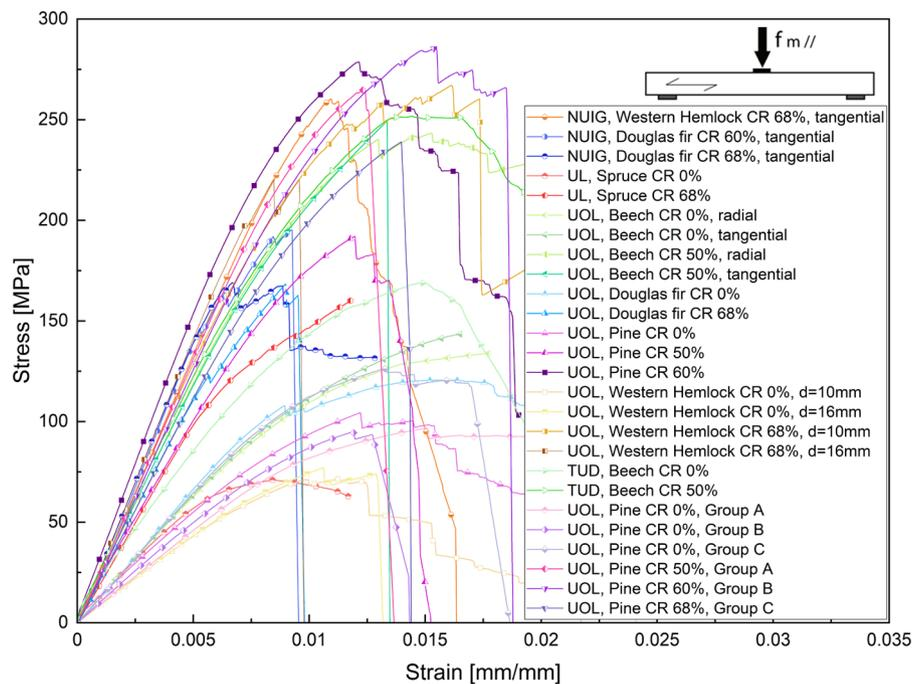
Fig. 8. Average stress–strain curves for bending tests.
