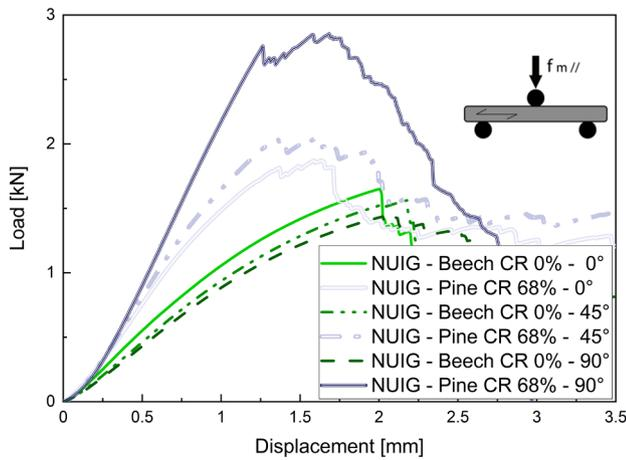
Fig. 10. Average load–displacement curves of yield moment tests.
