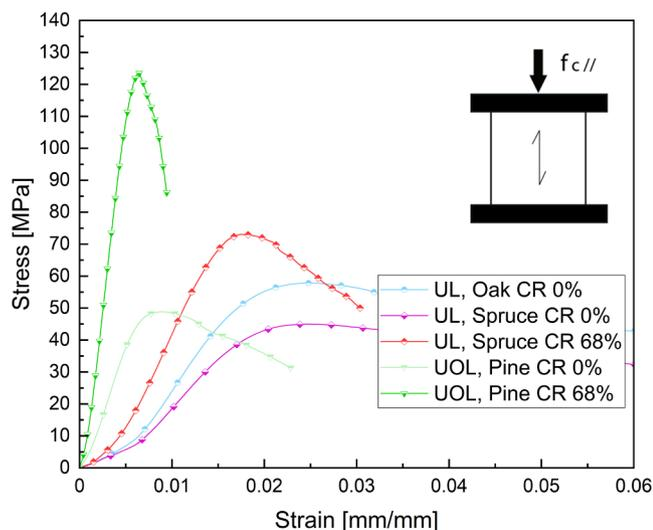
**Fig. 4.** Average stress–strain compression test curves in the longitudinal direction.
