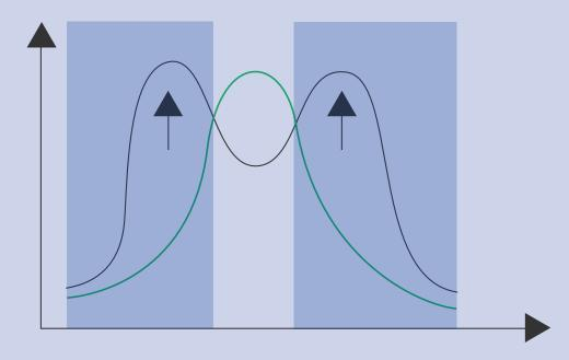
During blue moments (more demand than supply) the storage device can be set to discharging mode. This will result in an increase of supply.
