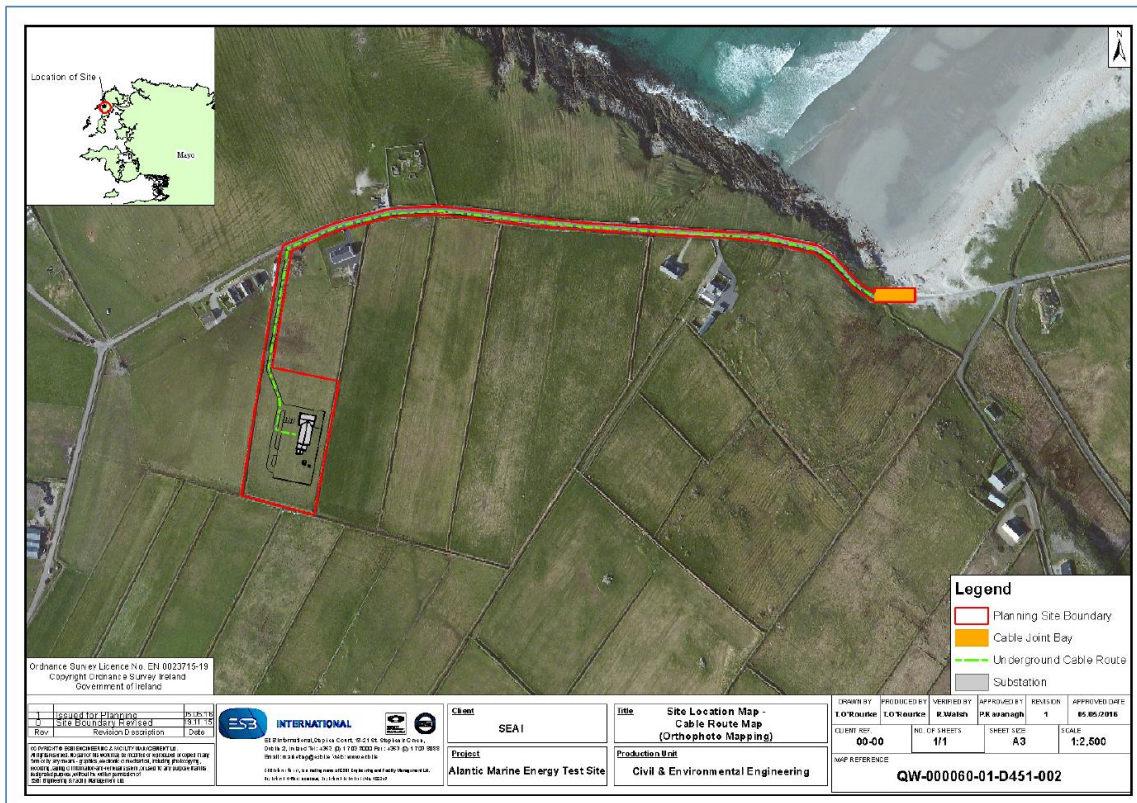
Figure 4. Export Subsea Power Cable Layout
