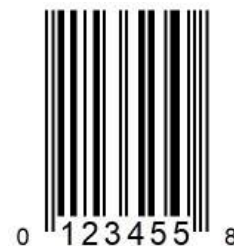
Figure 5.2.2.4-1. UPC-E barcode (encoding 001234000057 by zero-suppression)
