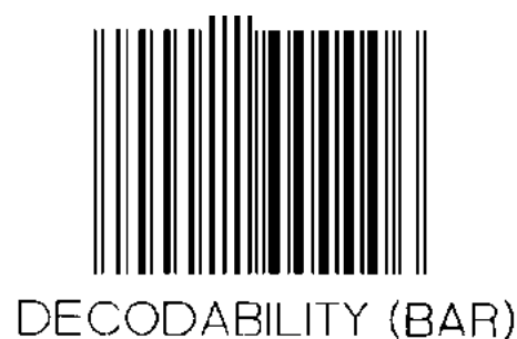
Figure 5.12.5.12-3. Calibration symbol with engineered low decodability grade
