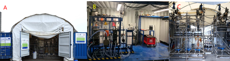
Figure 4: (A) mobile PULSE demonstrator (© Uliège-Michel Houet); (B) drying, leaching & precipitation modules (© Uliège-Z. Shariff); (C) mixer-settlers for solvent extraction (© Uliège-Michel Houet)
