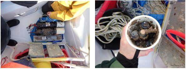
*Figure 3: Typical multisensory probe (see 4.3.10) with an internal colonization after 4 months even in presence of a brush. © F. Schoefs-Université/Capacités.*
