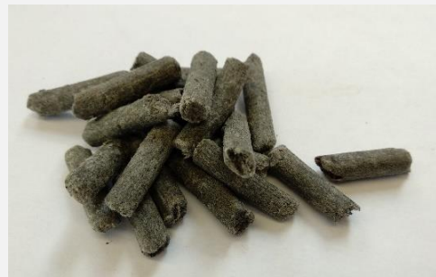
Cellulose Pellets Feedstock of the pyrolysis reactor
