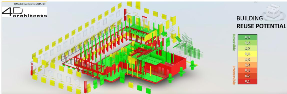
**Figure 5. Color coded Reversible BIM module (Durmisevic, 2020)**
