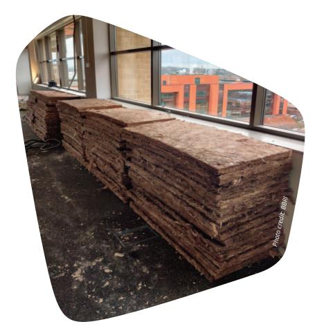
For example, the dimensions of panels of mineral wool can be measured directly, on-site or offsite. Other types of performance, such as mass density, squareness or flatness can be measured in the same way, with the evaluation of these performances only requiring limited equipment.
