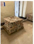
The growth for same site brick reuse was impacted by rigid programming as the brick removal, cleaning and reinstallation exceeded the construction timescales. The pilot coordinator challenged proposals to recycle the brick as hardcore, advocating reuse over recycling to minimise carbon-intensive processes on a brick that had structural integrity.
