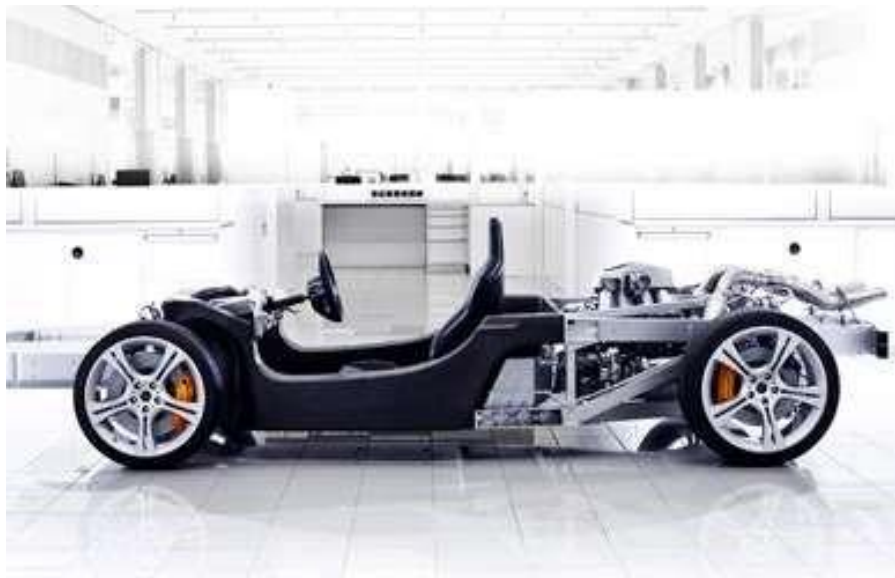
Fig. 7-3: The McLaren MP4-12C relies on the combination of carbon bathtub and aluminum subframes. Source: McLaren.
