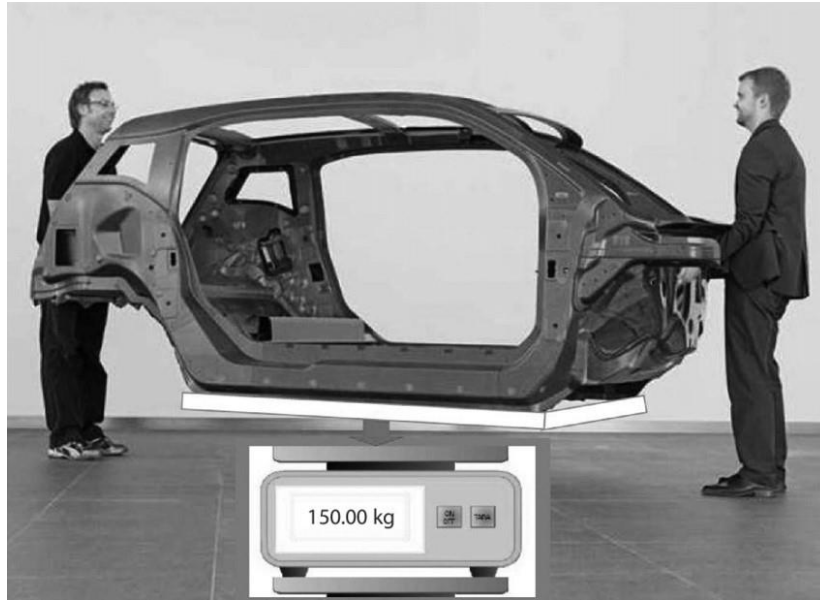
Fig. 6-10: Lightweight, carbon fiber-based composite life module of the BMW i3. Source: BMW.
