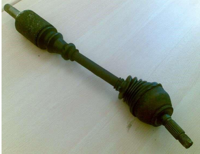
Fig. 6-1: A typical front-wheel drive CV axle
