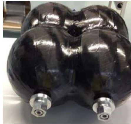
Fig. 6-13: A multi-spherical cryogenic vessel for H 2 storage: design, fabrication and testing.
