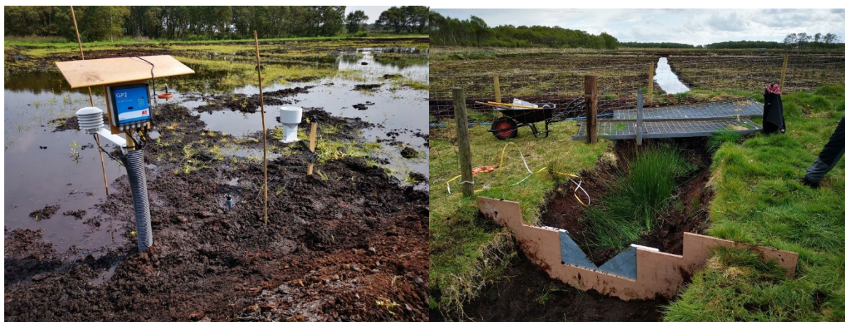
Figure 1: a) Meteorological station installed at Winmarleigh Carbon Farm and b) V notch weir installed with dipwell logging and autosampling to monitor DOC losses.
