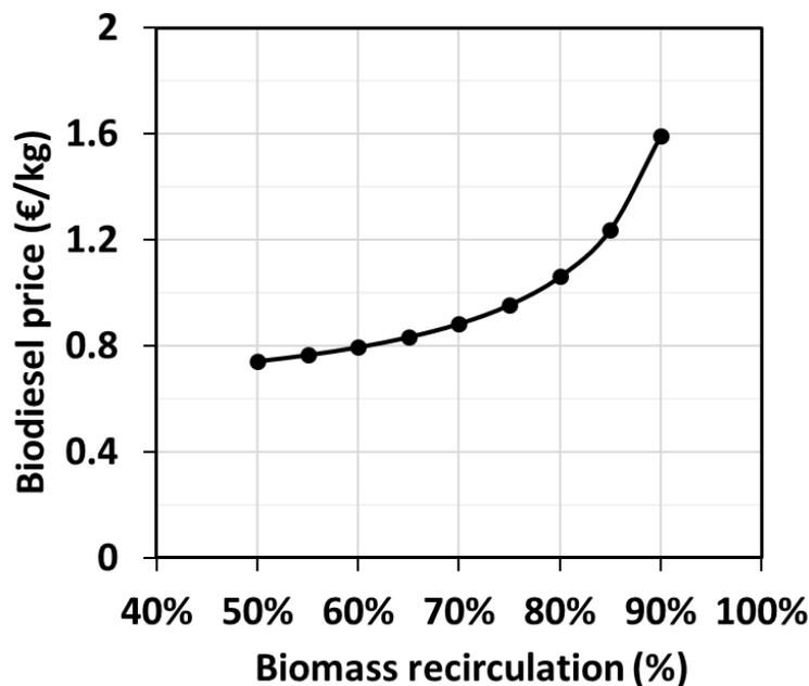
Figure 10. Impact of biomass recirculation on biodiesel MSP
