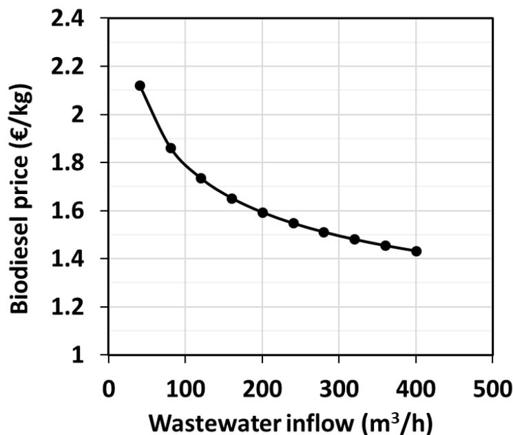
Figure 9. Impact of plant scale on biodiesel MSP
