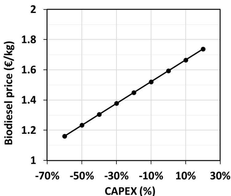
Figure 11. Impact of CAPEX on biodiesel MSP
