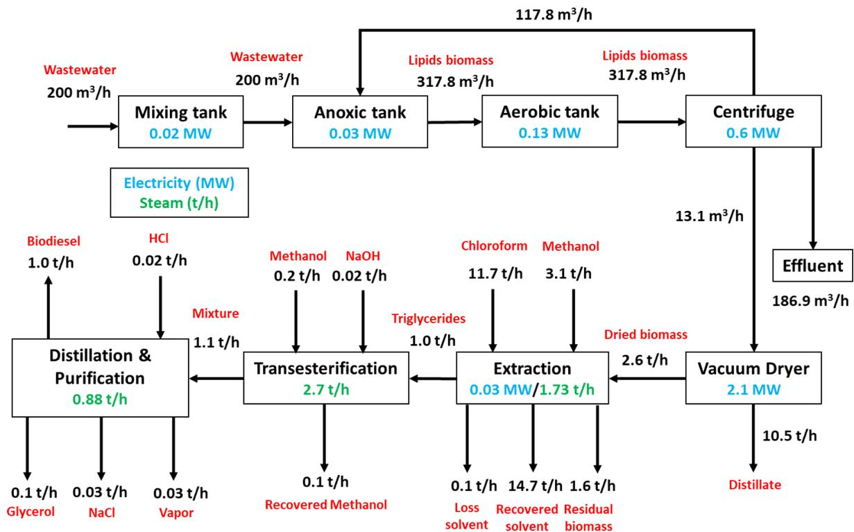
Figure 4. Mass and energy balance of biodiesel production
