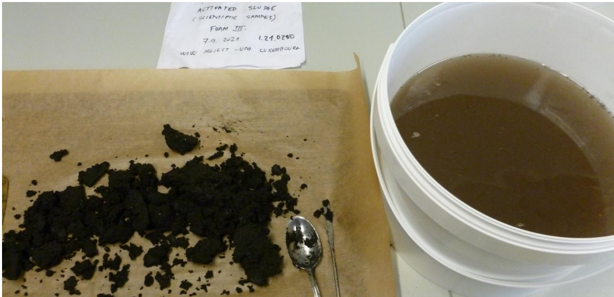
Figure 20: Separated Foam III material with sediment (left) and liquid (right)
