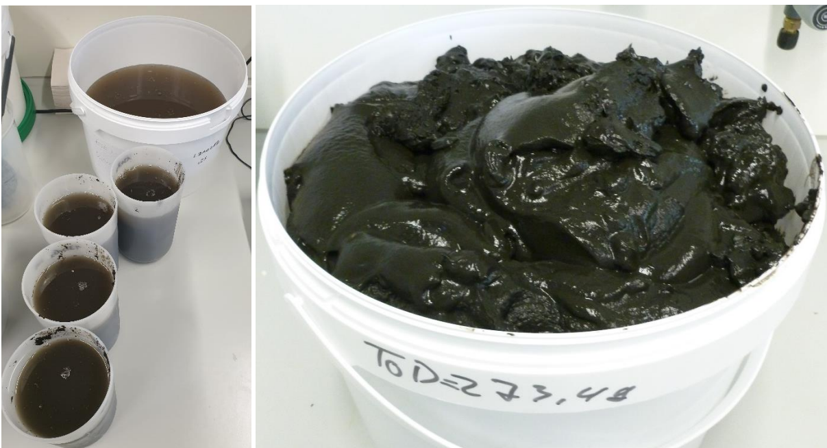
Figure 19: Activated sludge-foam in beaker for centrifugation (bottom of left picture), after centrifugation with liquid phase (top of left picture) and solid phase (right).
