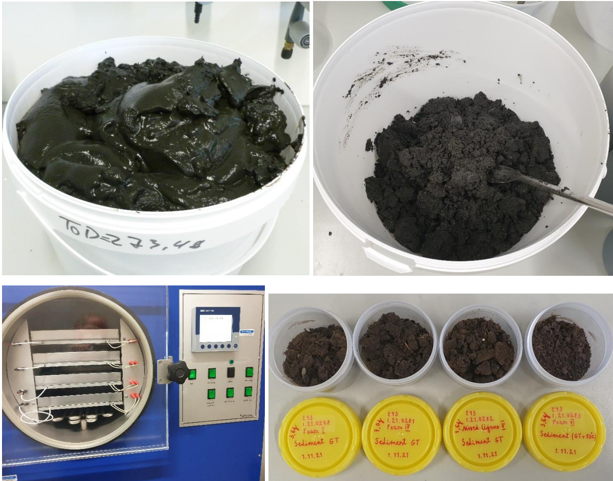
Figure 22: Concentrated sludge wet (left top) and dry (right top) sediment for freezing on plates, freeze drying (bottom left) and freeze-dried samples (bottom right).
