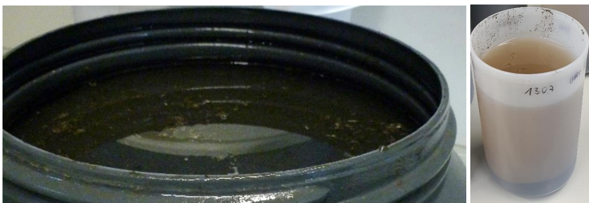
Figure 17: Material V mixed liquor before and after centrifugation.
