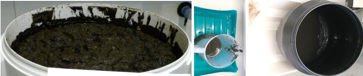
Figure 18: Activated sludge-foam before (left) and after freezing (right).
