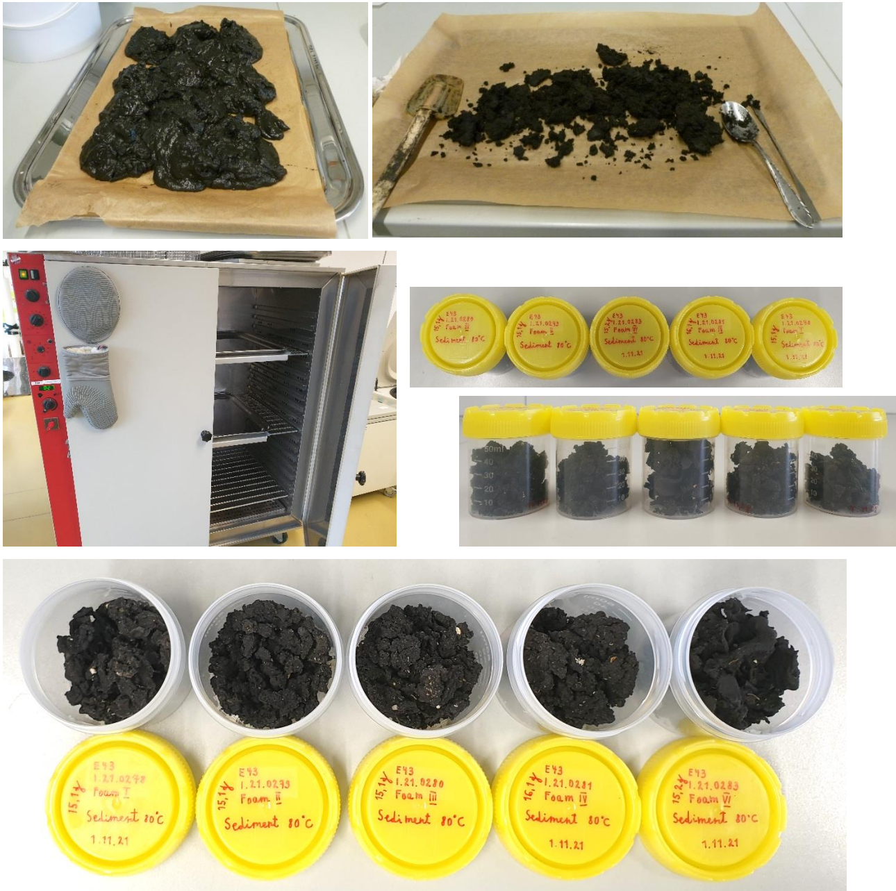
Figure 23: Activated sludge on a drying plate (top), Air drying oven (middle left), dried material (middle right and bottom).
