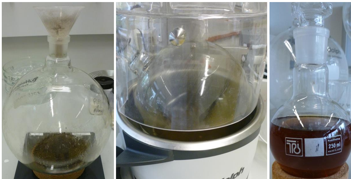
Figure 13: Extraction of fat from freeze-dried sewage slug.
