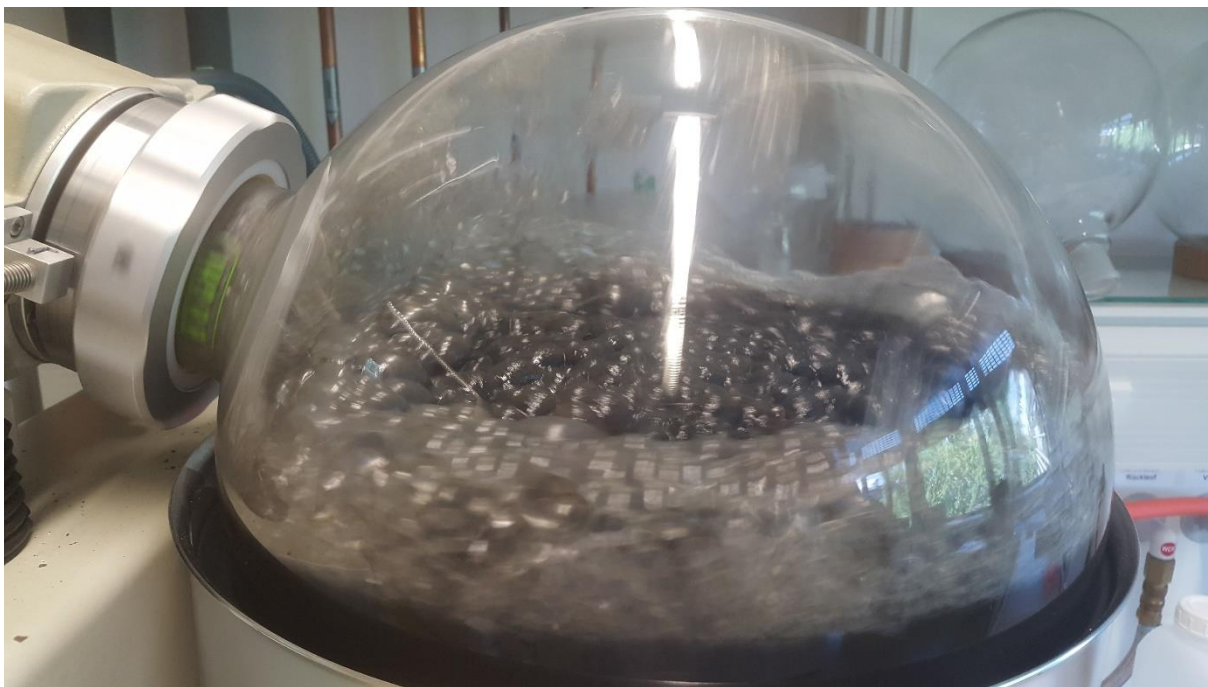
Figure 6: Material 31.05.2021 R1 during vacuum distillation. Strong foaming during reduction of pressure.
