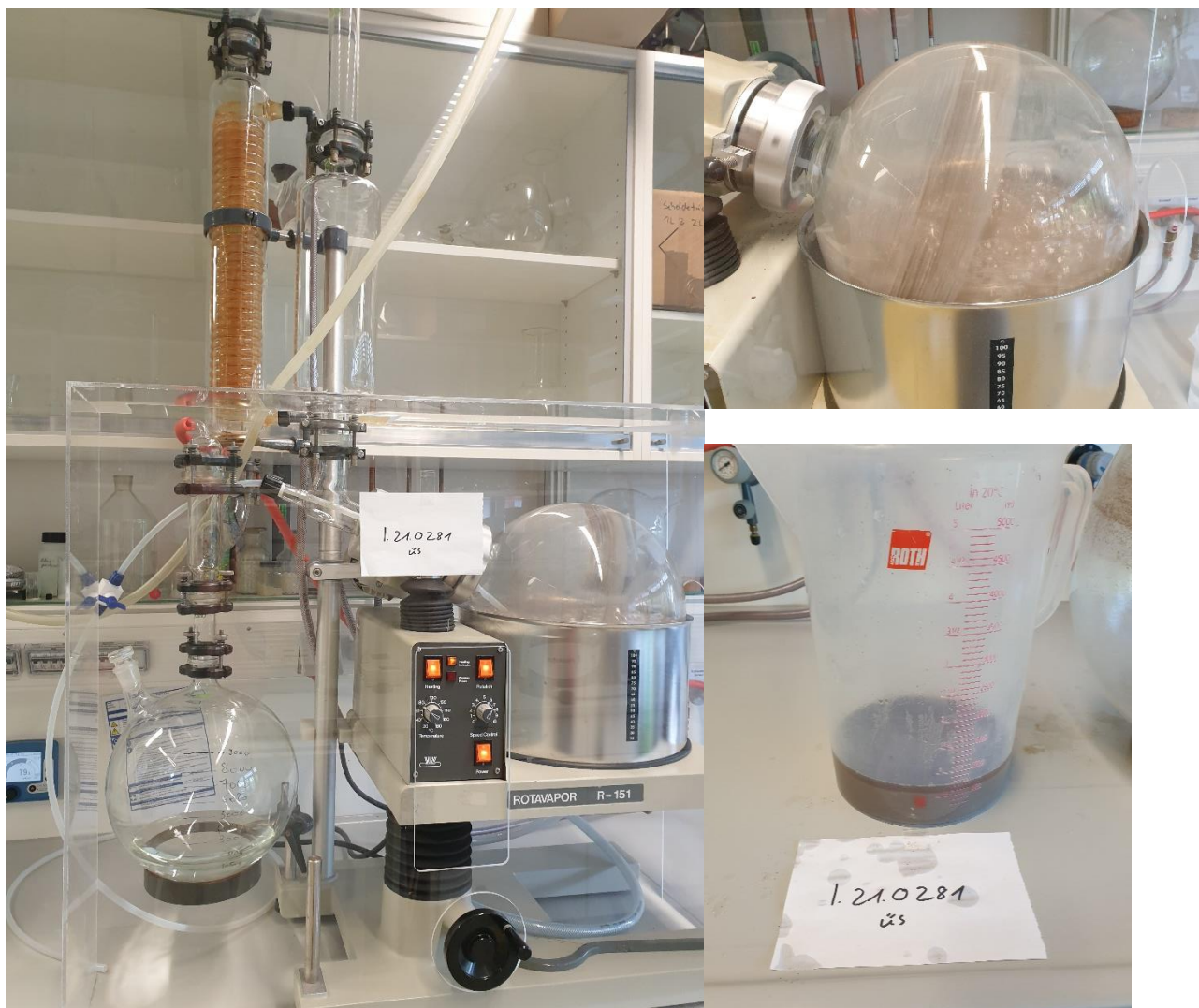
Figure 21: Concentration of the supernatant in a vacuum evaporator.
