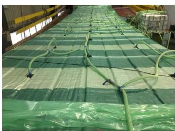
The bridge deck is manufactured as a complete element using a vacuum infusion process
