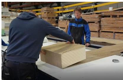
Production process: fibre mats made from flax are wrapped around light-weight foam cores.
