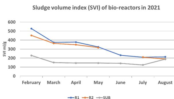
**Figure 7. Sludge volume index (SVI) monitoring at the Lipids-pilot plant in 2021.**
