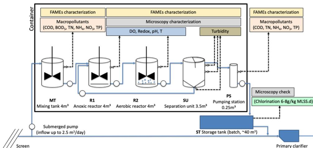
Figure 4. Schematic diagram of the pilot treatment system (Source: University of Luxembourg). The direction of the flow through the individual tanks is indicated by the solid blue lines, and sampling/sensors measurements, by the black dashed lines.
