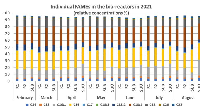
**Figure 16. Individual FAMES from the bioreactors at the Lipids-pilot plant in 2021.**
