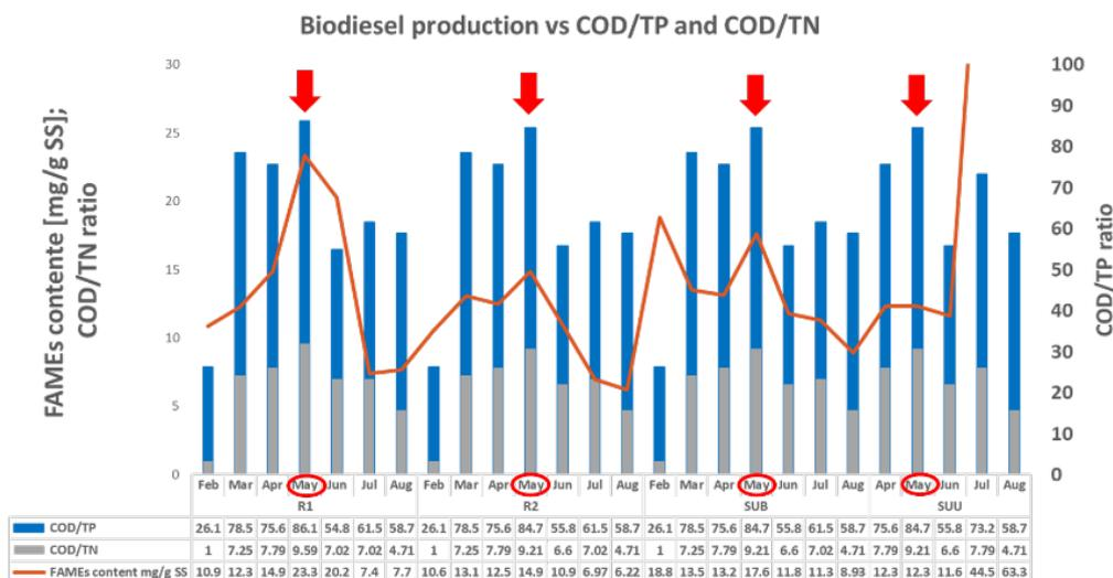
Figure 17. Comparison between Biodiesel production and COD/TN and COD/TP ratios of inlet wastewater in 2021.
