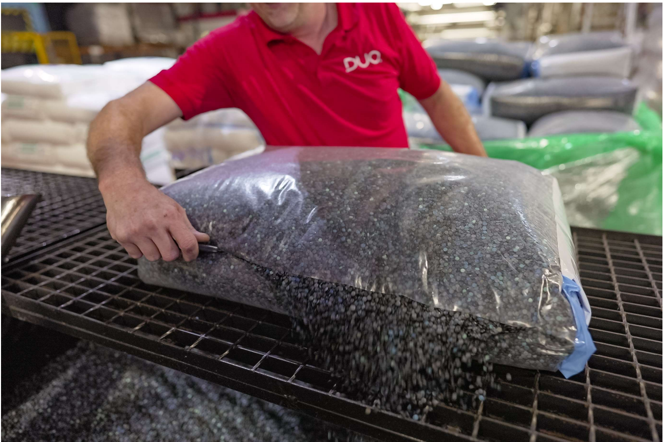
Figure 7: Recycled polyethylene pellet being blended on site at DUO.
