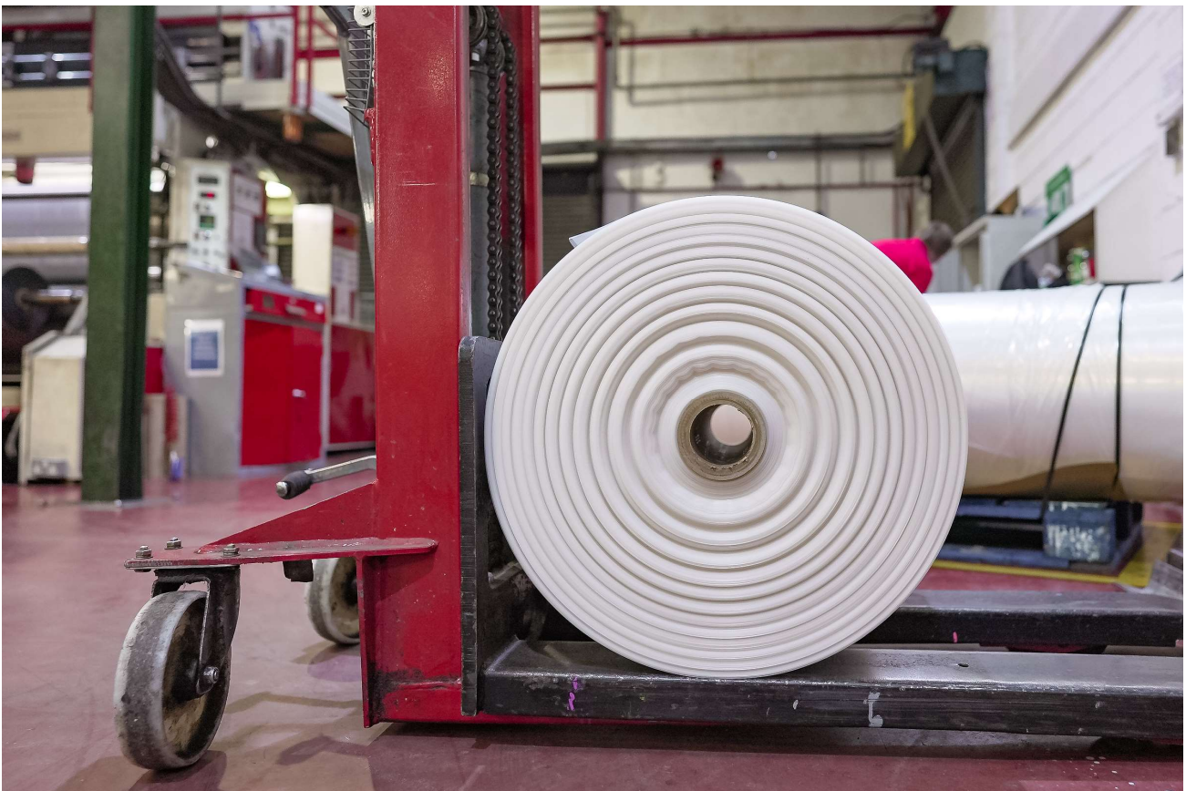
Figure 3: Film-blown extruded plastic awaits conversion into DUO's finished products.
