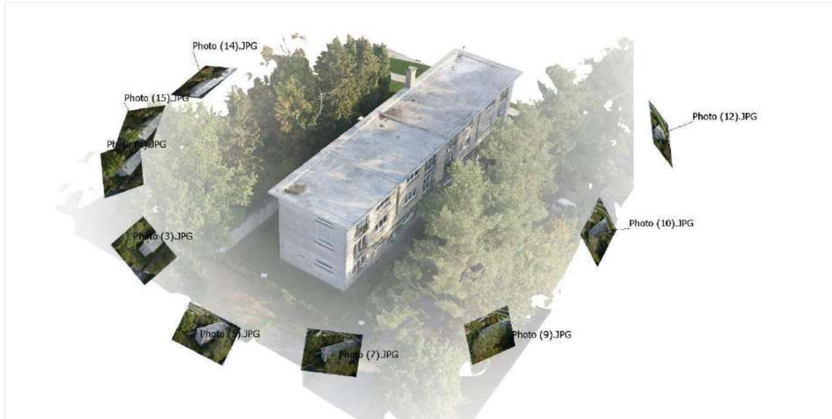
Figure 24. The principle of multi-view 3D reconstruction, or more simply called 'Photogrammetry' (source: BBRI)
