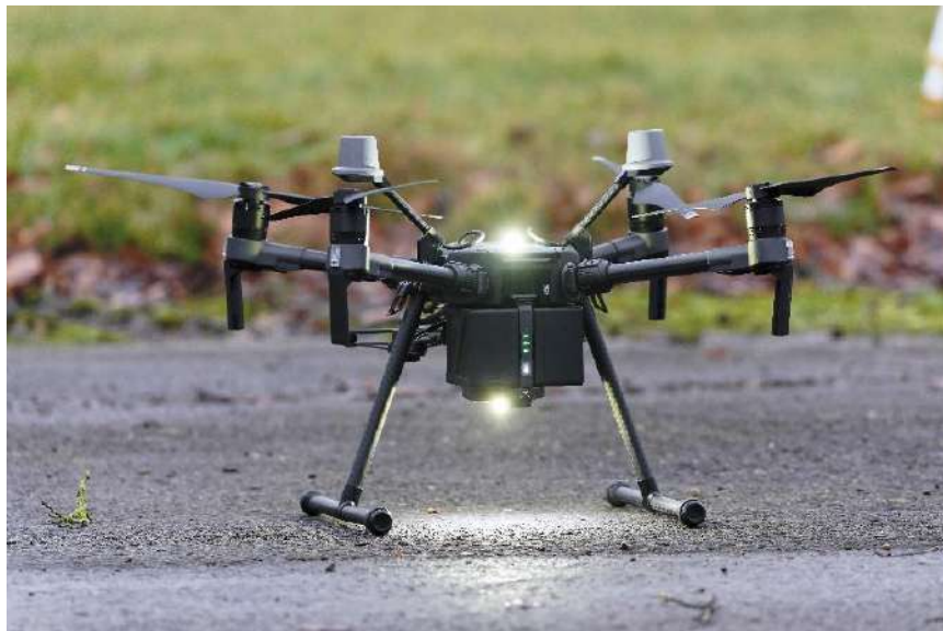
Figure 26. High-end drone equipped with a 'RTK' positioning system, providing highly accurate geotagging of pictures (source: BBRI)
