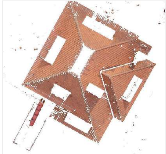
Figure 27. Segmentation of a point cloud based on colour information. Here the process was aimed at detecting tiles (source: BBRI)
