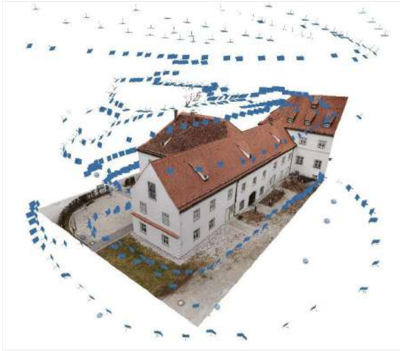
Figure 35. Scanning the 'Alte Schöfflerei' of the Monastery of Benediktbeuern.
