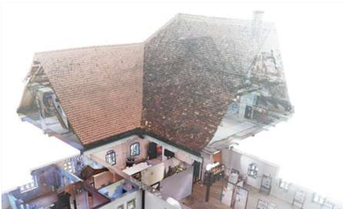
Figure 7. The XYZRGB point cloud, becoming one of the standard formats for high resolution 3D capture. (source: BBRI)
