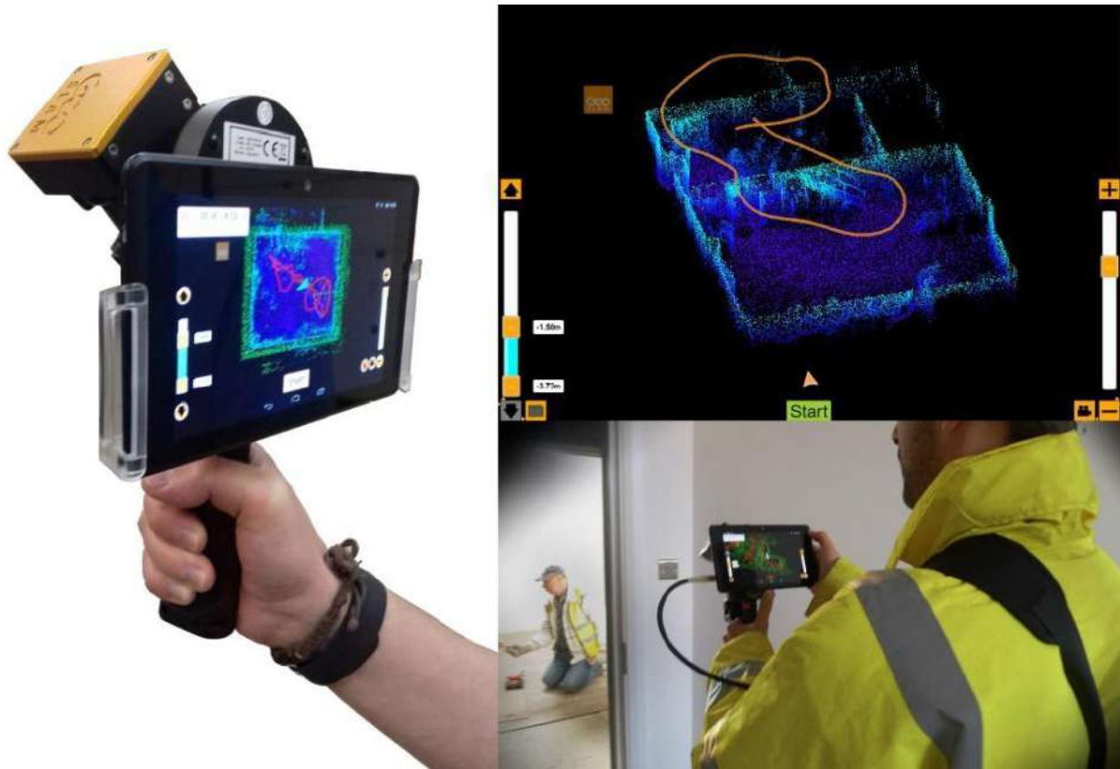
Figure 19. Point cloud from handheld SLAM (source: Geoslam)
