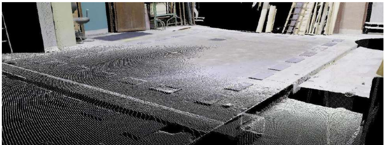
Figure 17. Loss of point density for objects at further distance from the scanner (source: BBRI)
