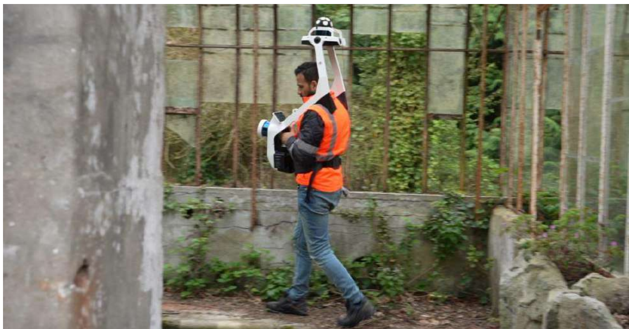
Figure 18. A mobile mapping system, carried on the back of the surveyor (source: BBRI)
