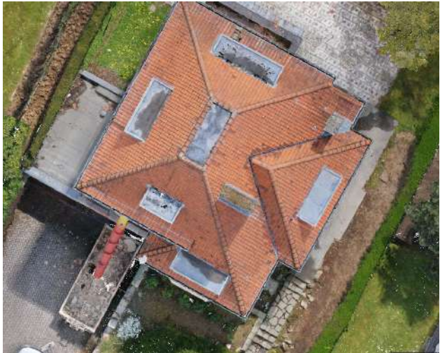
Figure 27. Segmentation of a point cloud based on colour information. Here the process was aimed at detecting tiles (source: BBRI)
