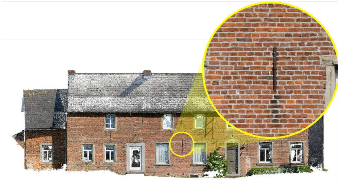
Figure 31. Orthoview of a façade, generated from a point cloud (source: BBRI)
