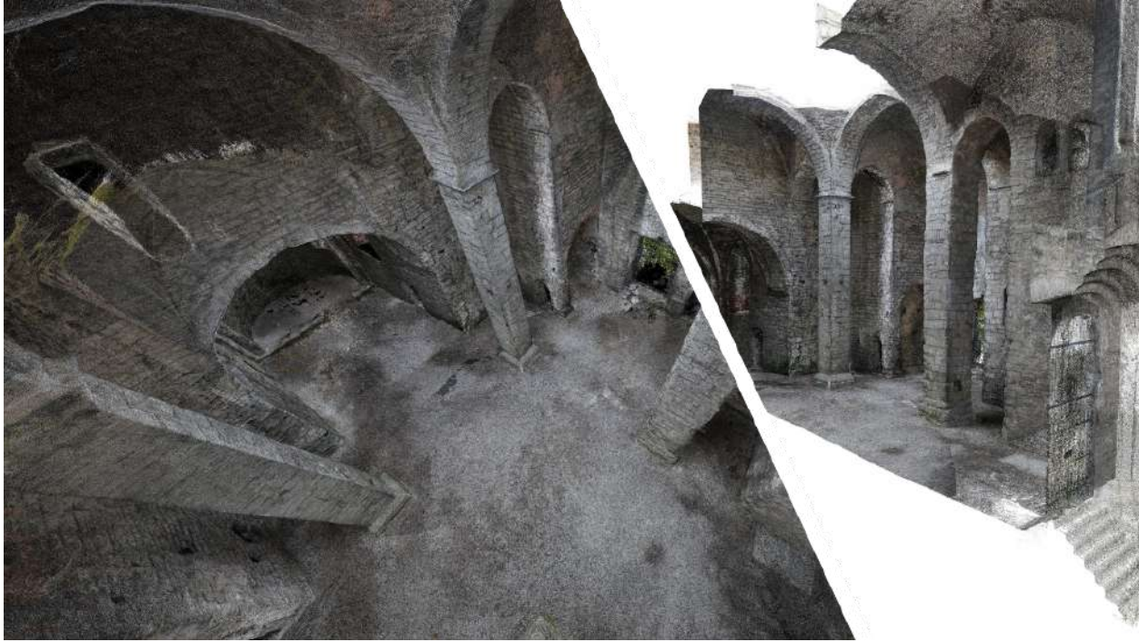
Figure 25. Photogrammetry is common in the Heritage sector, where highly textured buildings are found. It is legitimate to question the relevance of photogrammetry for more modern objects (source: BBRI)
