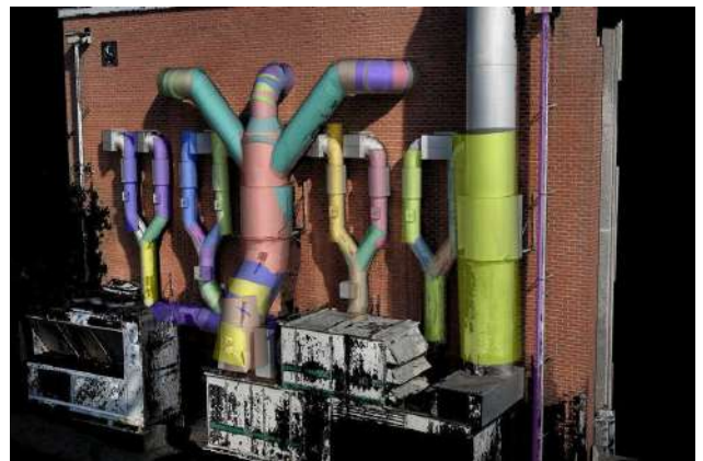
Figure 29. Cylinder shape detection using the RANSAC algorithm (BBRI)
