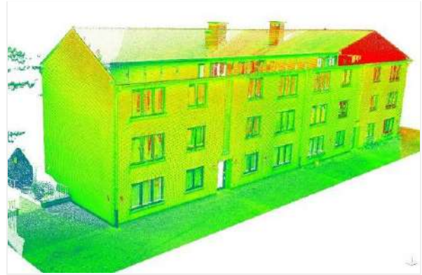
Figure 16. Intensity value mapped on the point cloud (source: BBRI)
