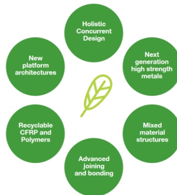
Figure 6: Key technologies driving lightweighting opportunities for automotive applications 102
