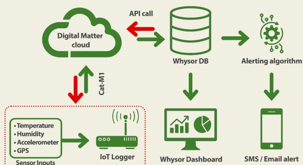
**Alerting logic.** The threshold values for the alerting system are defined by the technical team at Biogros, for all locations inside the warehouse or inside the truck. Text messages are sent if the limit value is exceeded, e.g., above 8°C in the vegetable department or above 10°C inside the truck.
