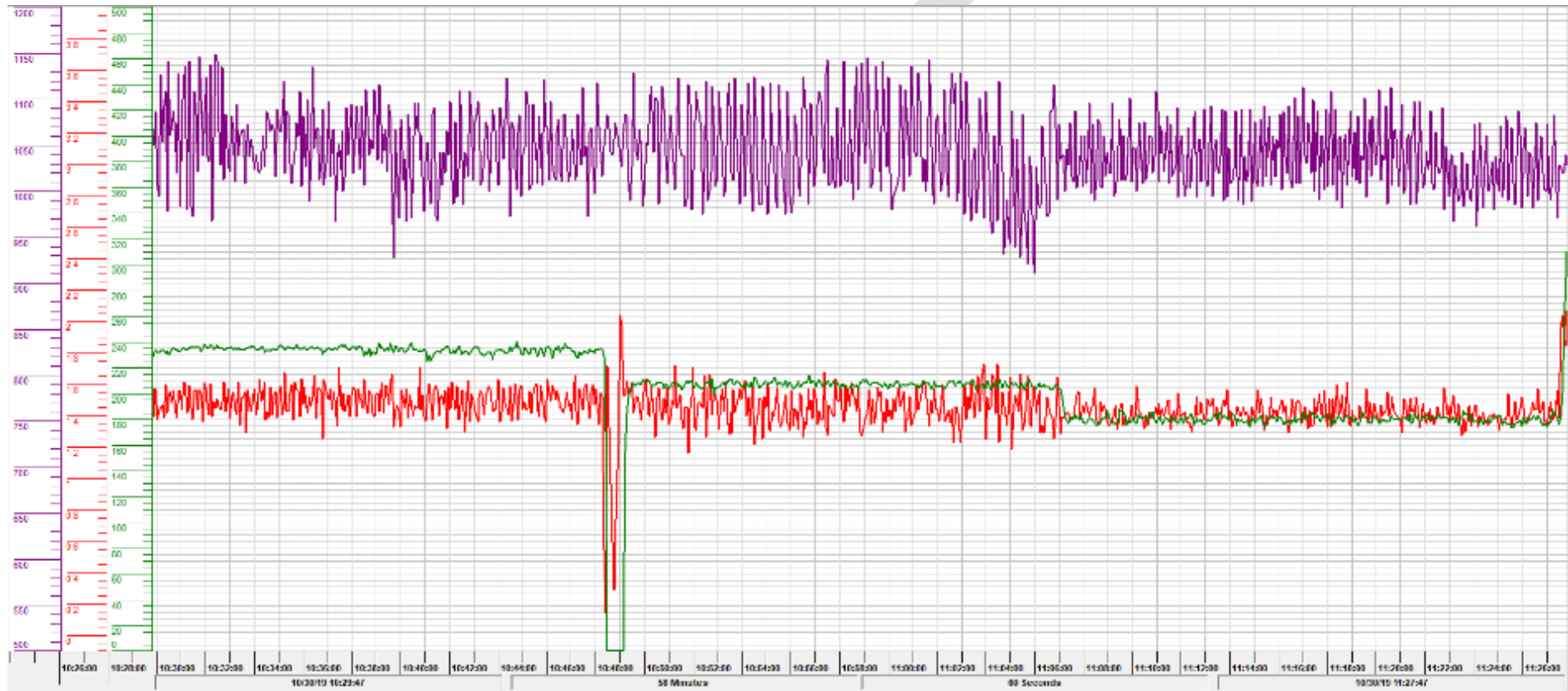
Figure 18 - Site Audit Measurement Trends for P2 only running at various frequencies (50Hz/47.5Hz/45Hz)
