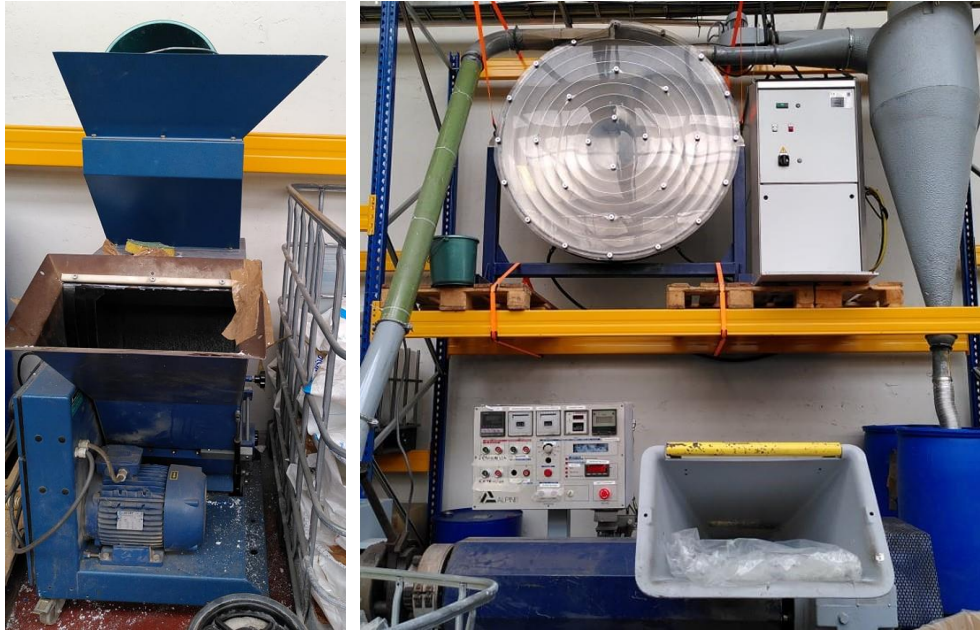
Figure 8: Shredder (left) and extruder (right) for waste pre-treatment
