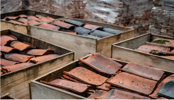
Roof tiles recovered manually, cleaned, packaged and stored, ready for reuse.
