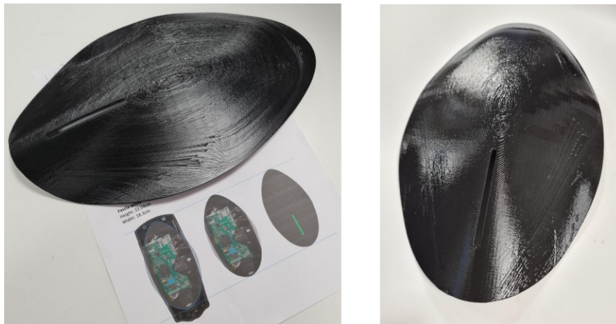
Figure 6: Final prototype before (Left) and after (right) vapor smoothing.
