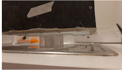
Adjusting kit on the outside of the seam decreased the water leakage
