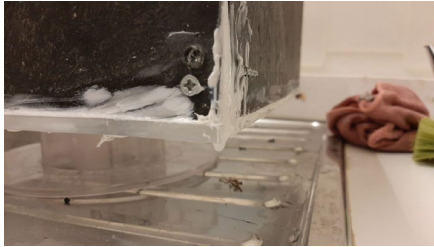
Adjusting kit on the outside of the seam decreased the water leakage
