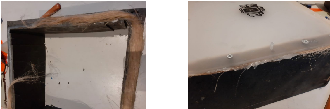
Screwing the bottom of the box on the sides with flax and Vaseline
