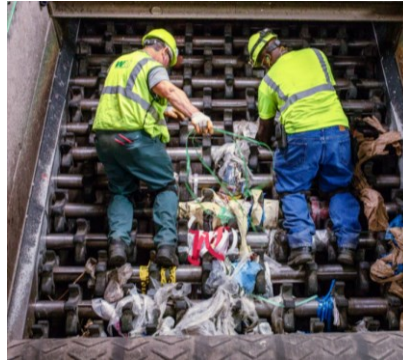
Figure 10 Workers removing thin plastics from a clogged disk sorting machine
