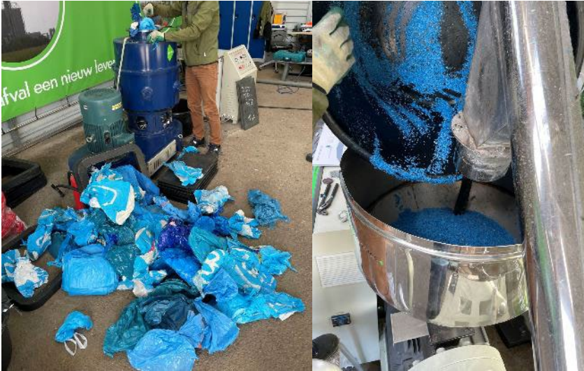
Figure 12: Blue bags as input material (left) and agglomerated pieces (right)
