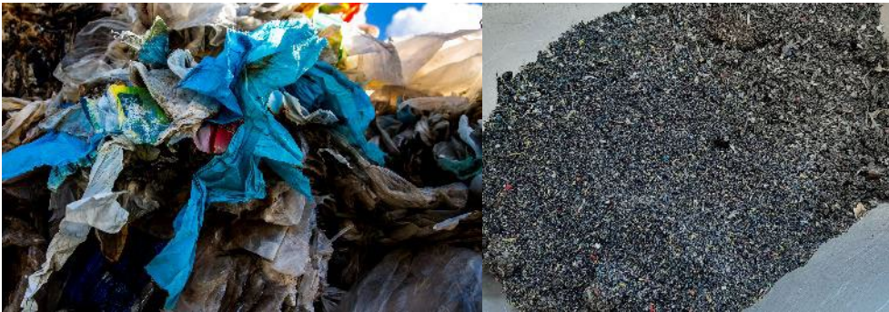
Figure 7: Input material at the Green Plastic Factory: mix plastic packaging waste (left) and agglomerated material (right)
