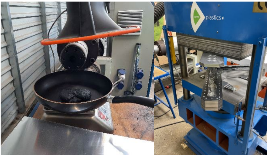
Figure 8: Extruded material (left) and pressing L-element (right)
