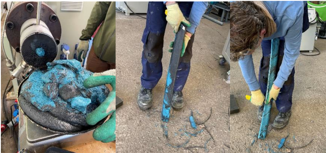
Figure 13: Molten material with two colours as input material (left) and finished bar (right)
