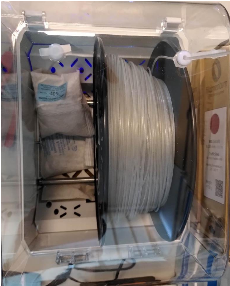
Figure 3: rPMMA filament from show-room glass lenses
