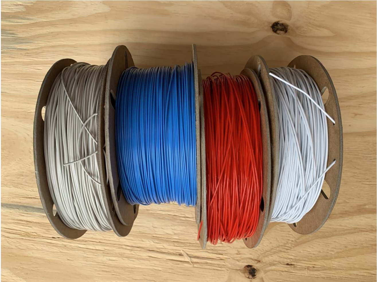
Figure 3: Spools of recycled 3D printing filament made via extrusion processes using 3D printing waste.
