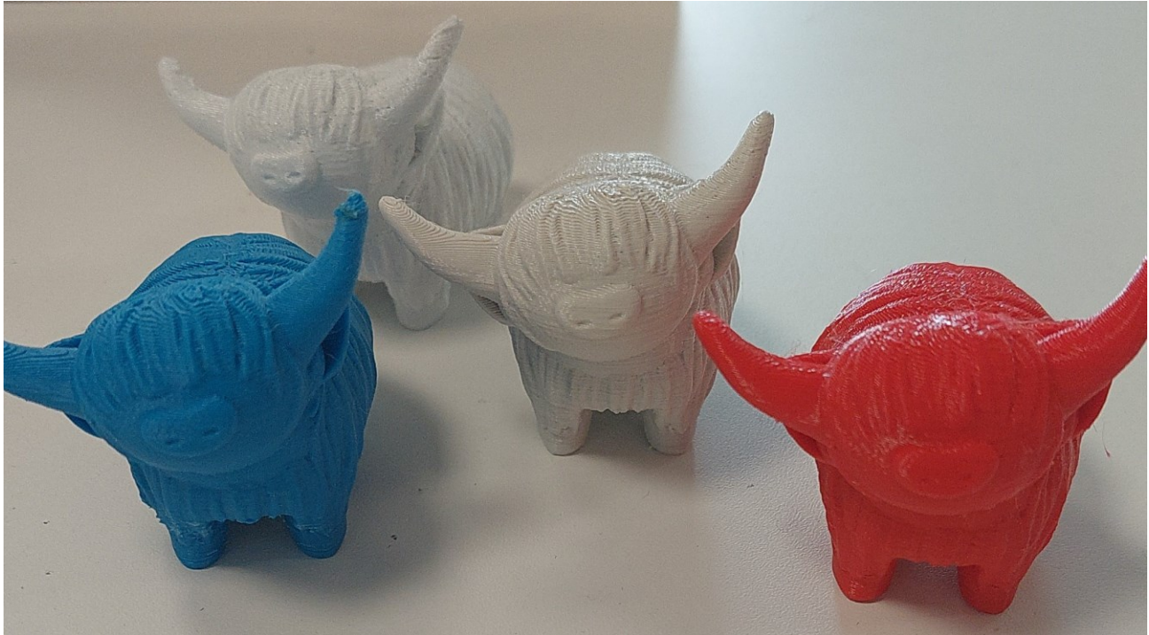
Figure 4: Test prints using recycled 3D printing filament.
