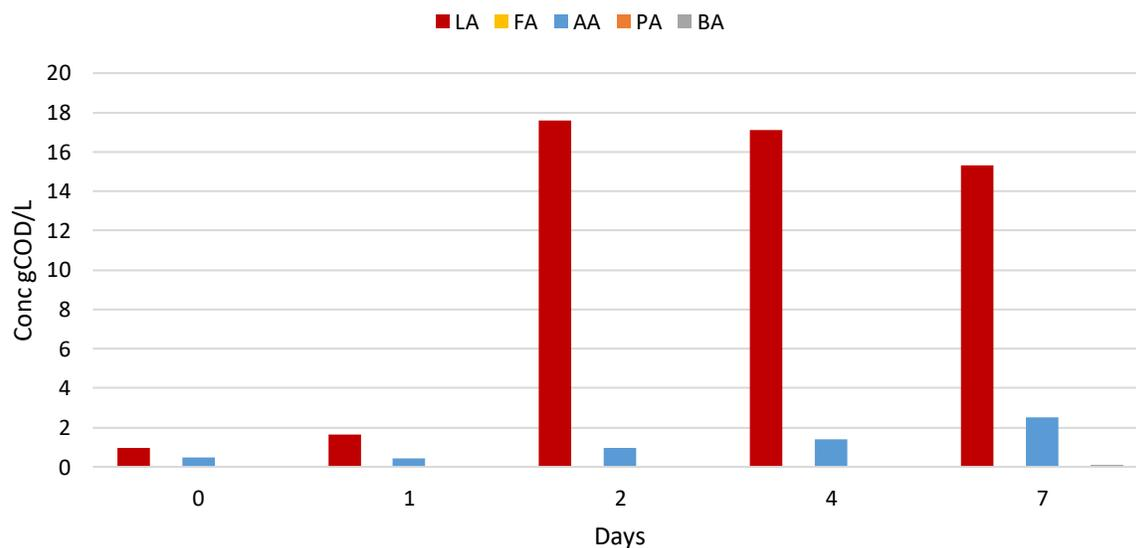
Figure 7: Profile of VFAs concentration during time for OP acidification
