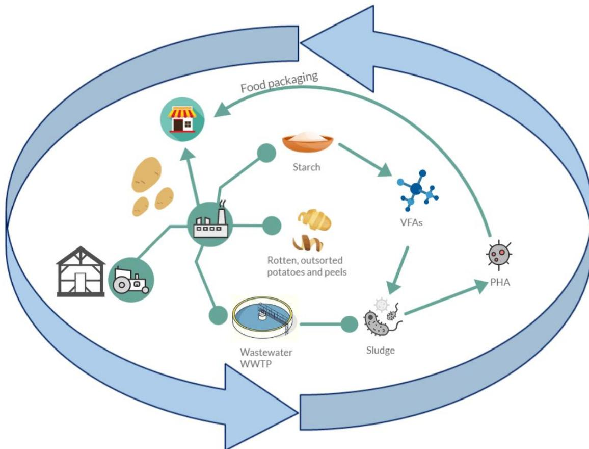
*Figure 1: Schematic representation of integrated PHA production in potato processing industry.*
