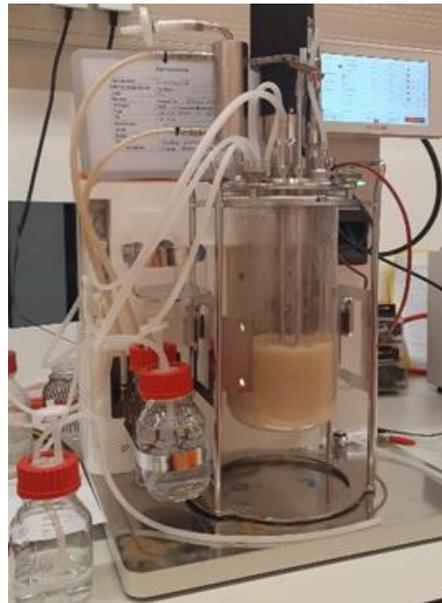
Figure 3: Bioreactor in anaerobic fermentation
