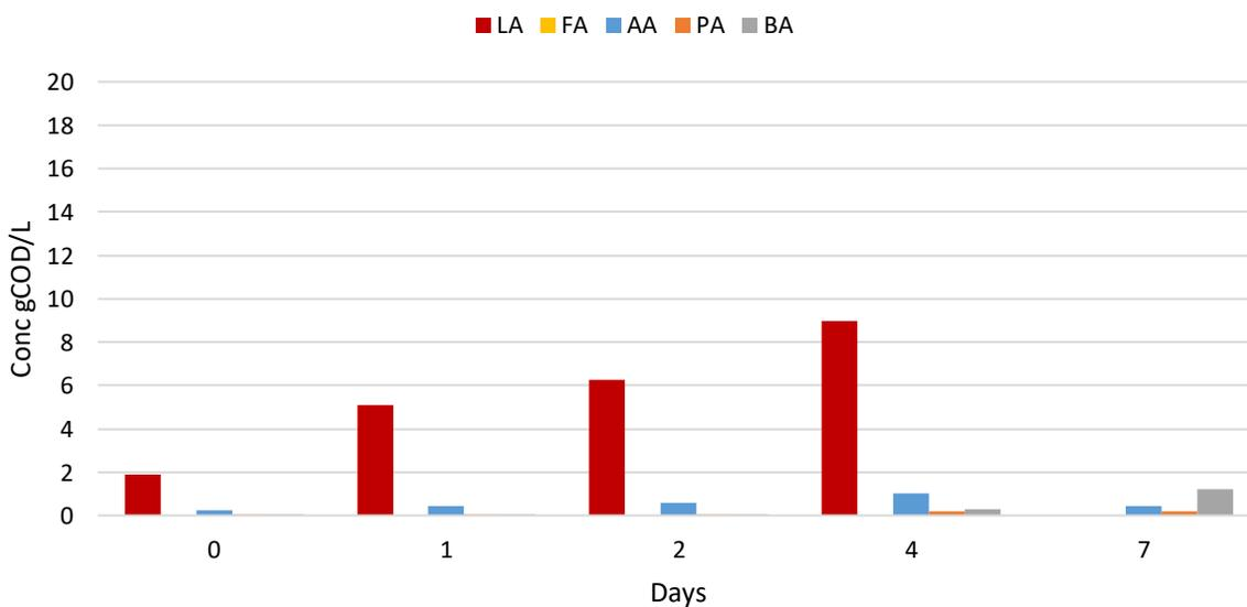
Figure 6: Profile of VFAs concentration during time for Spezial acidification.
