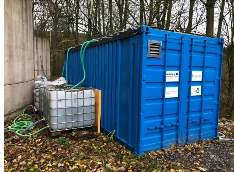
Pilot plant installation for PHA production
