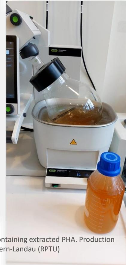
Figure 3. Filtered DMC solution containing extracted PHA. Production from the University of Kaiserslautern-Landau (RPTU)
