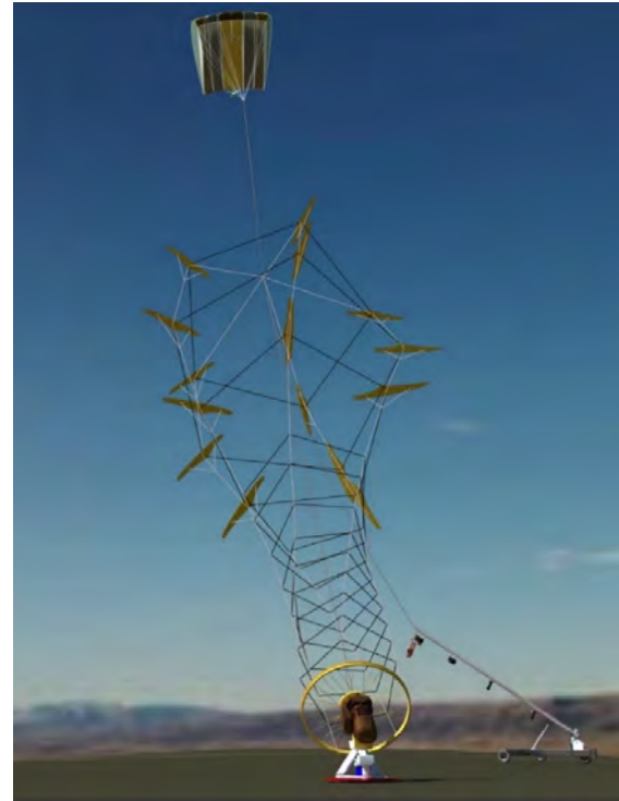
Figure 22 Ground-generating rotary device design.
