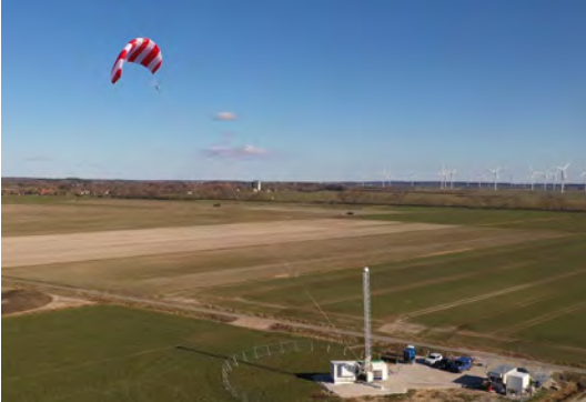
Figure 4 Ground-generating – reeling tether kite (Source: SkySails)
